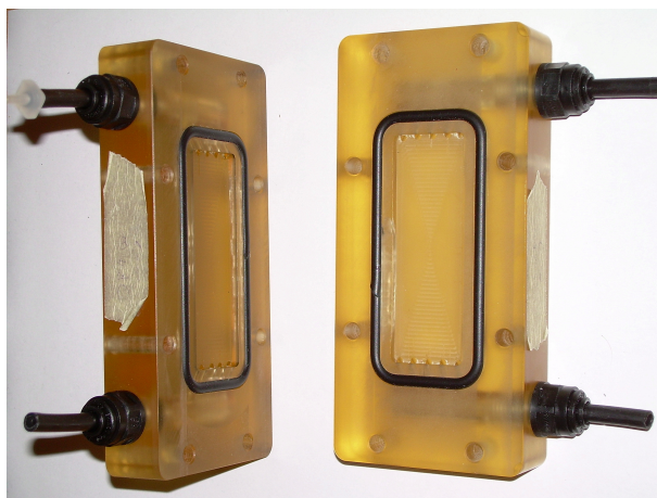
Figure 3.3: FO cell with the two channels for draw and feed solutions.
