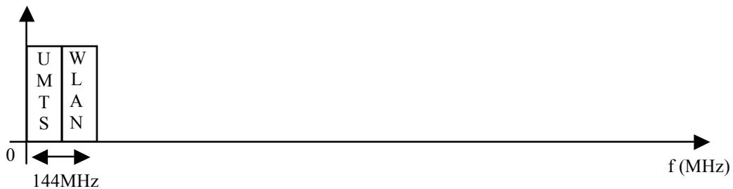
c) Input signal is brought to baseband by means of heterodyning. The spectrum occupation is now 144MHz.
