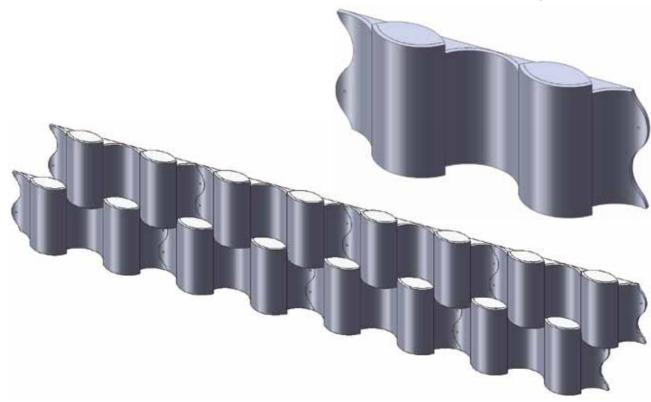
This version has only one outward curve instead of two. This was done to increase the volume of the foam. However, the aesthetics suffered under this and the idea was deselected. The two outwards curves were therefore reselected.
