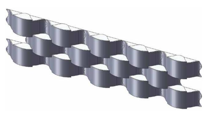
Even if the two outwards curves was to be kept, there were still problems with the ends of the wave. The curved ends did not seem right and there was only one possibility of letting the waves intersect. The curves at the ends are not actually necessary and the ends themselves were in fact blocking an opportunity for letting the waves intersect in more ways.
