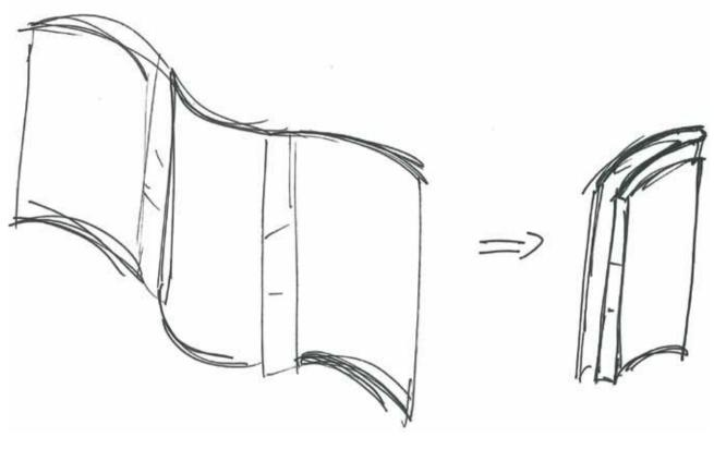
The sketch above shows an idea for a foldable screen that by its curve also has a modular built that allows it to be put together with other screens.
