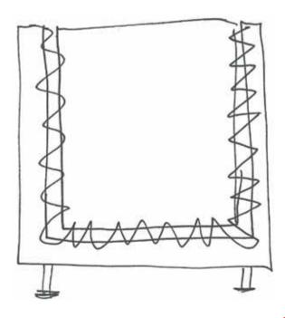
The sketch below shows an idea for a shelving unit produced in gas concrete, which with its open surface has a noise reducing effect.
