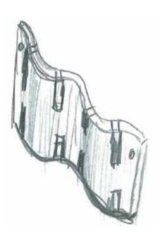
The sketch below shows an idea for the divider screen design. The design consists of two layers: a thinner layer of hard felt to keep the shape and a thicker layer of foam to absorb the low frequencies. The design is circular to obtain better stability and to diffuse the noise that is not absorbed. On the top and bottom edge it has cut outs to let two or more items intersect as a sort of puzzle.
