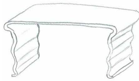
The sketch to the left shows an idea for a table clad in felt or similar to absorb and with a shape to diffuse the noise.
