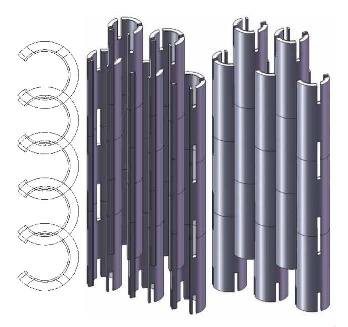
For the second version of the tube the intersection was made much shorter but the tubes were placed closer together. This construction made it possible to place a small plate inside a tube resting on an intersection thereby creating a small shelf. However, even though the shelf worked, it was too small and the access to it was even smaller; a grown man could barely fit his hand in through it. Therefore the entire tube idea was deselected.
