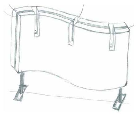
Another transparent gel idea is shown on the sketch below. Here the gel inserts are placed at the top of the screen to allow more light to penetrate the screen. The screen has also received a wave shape that diffuses the noise not absorbed by the screen.
