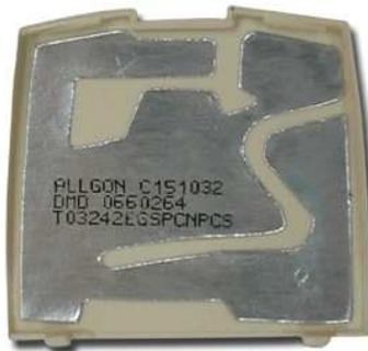
Figure 3.3 : PCB antenna
