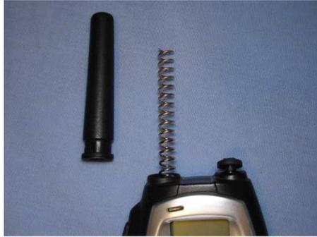
Figure 3.2 : Coil antenna
