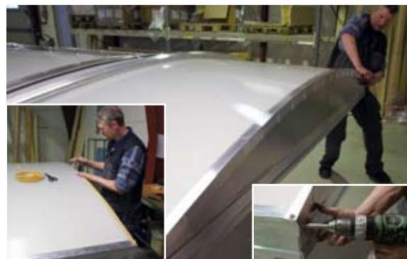
[ 26 ] Self-adhesive rubber lists are applied on top of the fixed PC plates at each end of the skylight. Vaulted alu profiles are mounted on top of the rubber lists.
