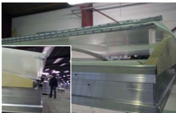
[ 14 ] Two PC plates are placed on top of each other on each side of the opening module. The PC plates are closed with tape that allows condensation to exit the ducts.
