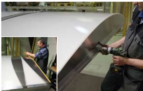
[ 25 ] Vaulted alu plates are equipped with self-adhesive rubber lists and mounted to the wooden endgables.
