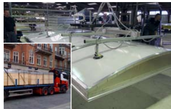
[ 27 ] The assembled PC light is lifted outside for storage until transport to the customer.
