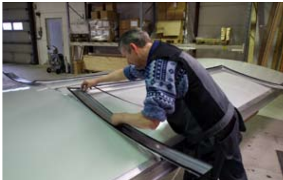
[ 19 ] Two welded alu profiles - to ensure the openings between the modules are tight when the window is closed - are equipped with self-adhesive rubber lists.
