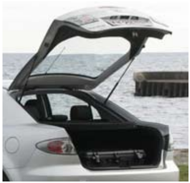
ill. 2.16. - Tailgate on a car with pneumatic actuators and a weather strip round the border on the hatch.
