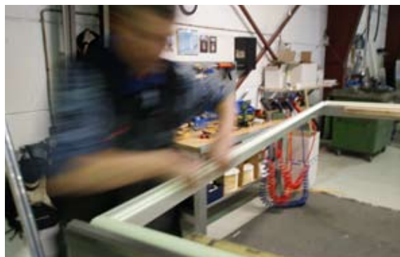
[ 8 ] Plastic lists are clicked onto the two short sides of the alu frame.
