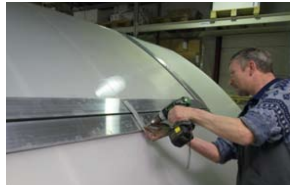
[ 21 ] An alu profile is mounted between the two opening modules to ensure the window can't open during transport. (Profile is removed during mounting)
