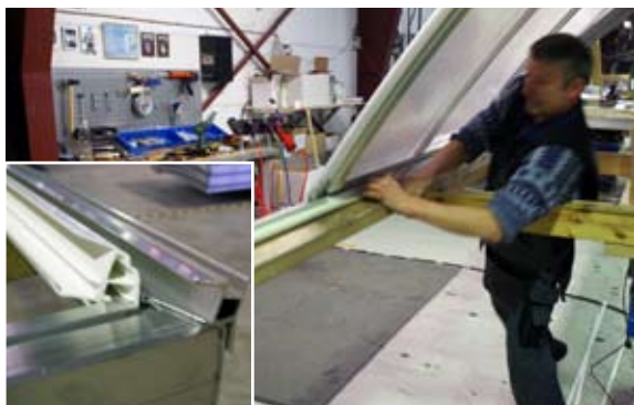
[ 7 ] The plastic profile is clicked on to the alu frame in the full length of the long sides.
