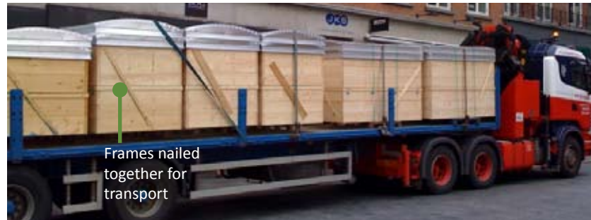
ill.3.71 - Pre-assembled skylights on a truck packed in a bundle of two. Two frames are nailed together on top of each other and two window modules on top of that.
