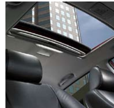
ill. 2.15. - Car sunroof that can slide away on tracks in the roof.
