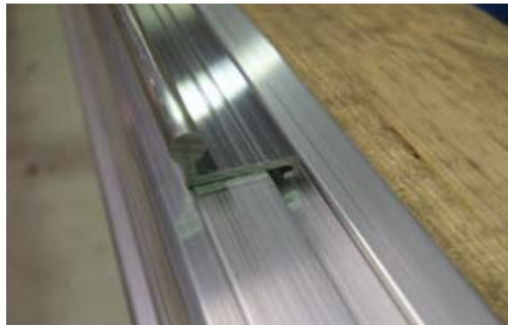
[ 2 ] An alu profile with a hinge for the opening windows is screwed onto the alu frame in the middle of each long side.
