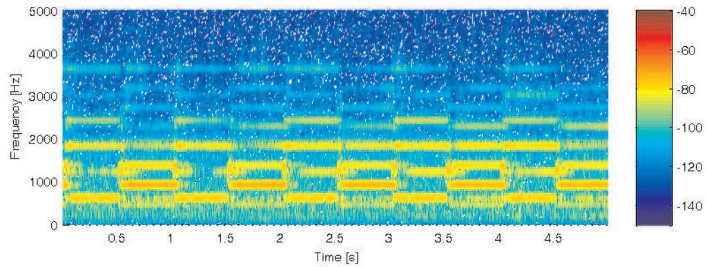
**Figure 3.13:** Spectrogram of the noise measured in the cabin when the ambulance is stationary and siren 2 is turned on. Note the duty cycle of siren 2 is seen.
