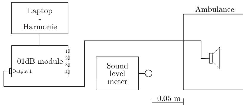
**Figure C.4:** Measurement setup for the facade leakage measurement.
