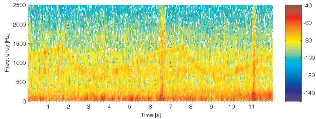
**Figure E.11:** Noise measured in the cabin when driving on highway with siren 1 turned on.
