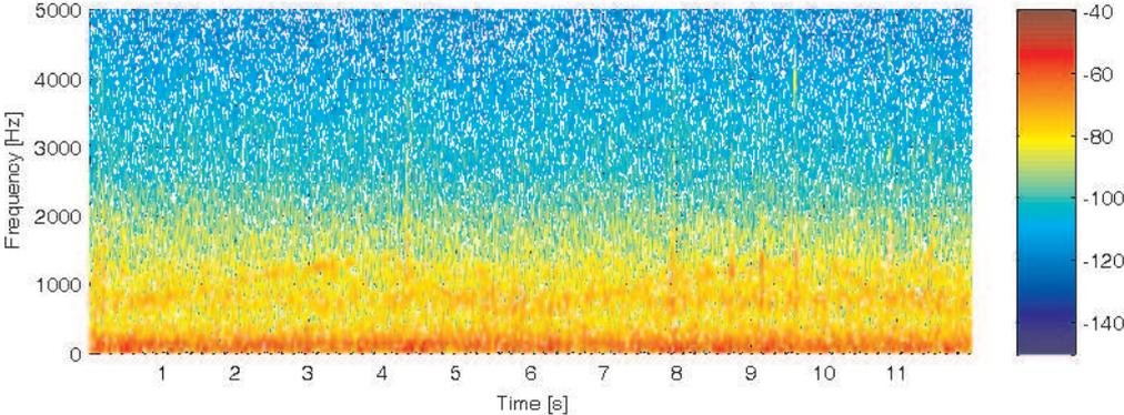
**Figure E.8:** Noise measured in the cabin when driving in on the freeway with siren 1 on.
