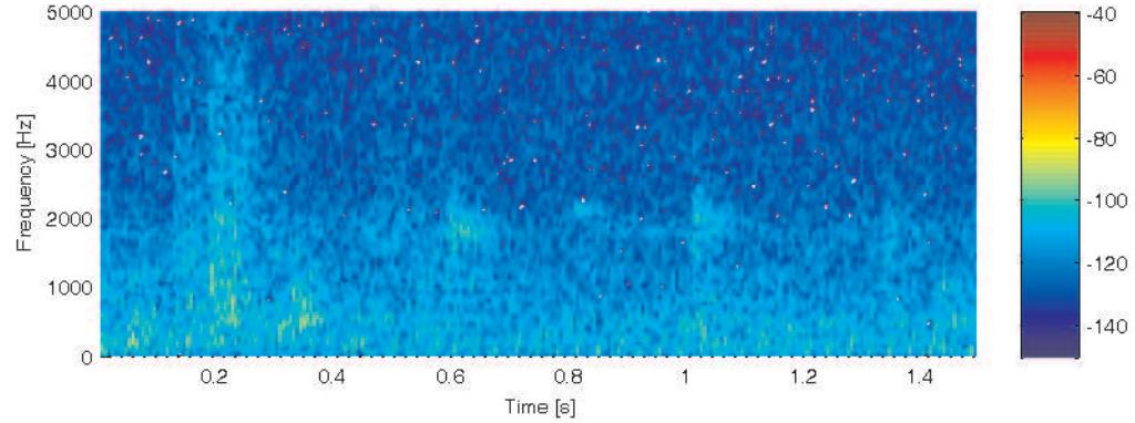
**Figure 3.14:** Spectrogram of the noise measured in the cabin when the ambulance is stationary and siren is turned off.
