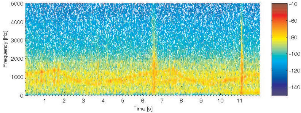
**Figure 3.20:** Spectrogram of the noise measured in the cabin when the ambulance is driving on the highway with siren 1 turned on.
