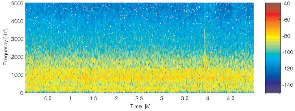
**Figure 3.22:** Spectrogram of the noise measured in the cabin when the ambulance is driving on the highway with the siren turned off.
