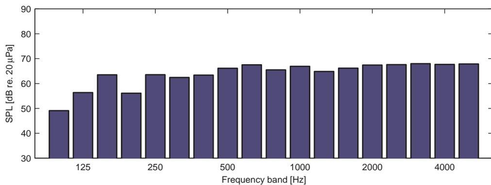
**Figure D.5:** Measured SPL in one-third octave bands from closing the rear right door of the ambulance.
