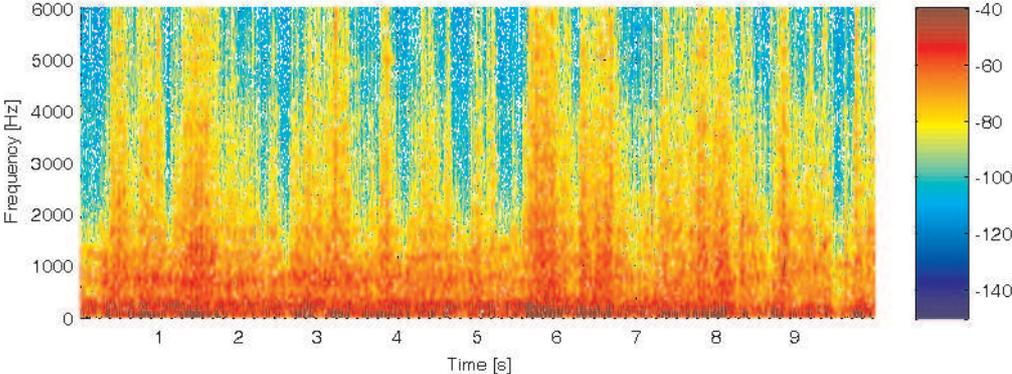
**Figure E.3:** Noise measured in the cabin when driving in the city with siren 1 on.
