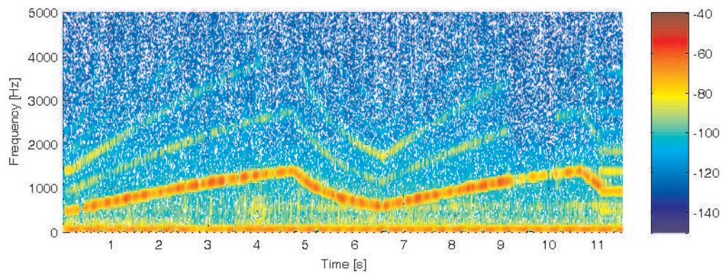
**Figure E.5:** Noise measured in the cabin where the ambulance is stationary and siren 1 turned on.
