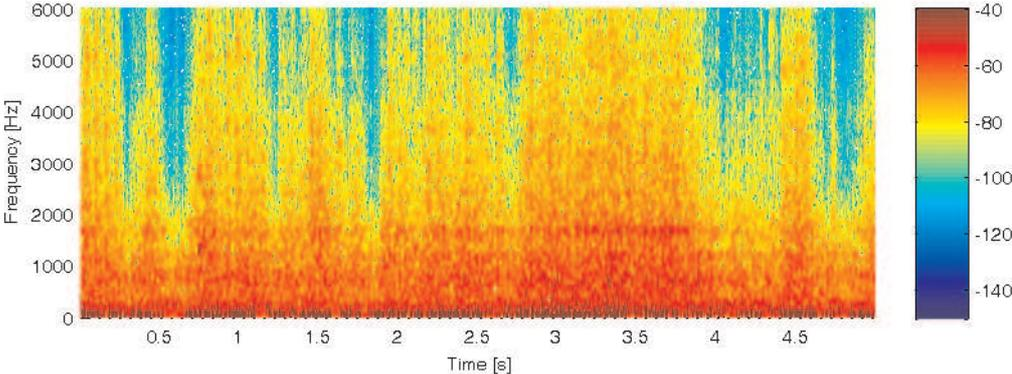
**Figure E.4:** Noise measured in the cabin when driving in the city with siren 2 on.
