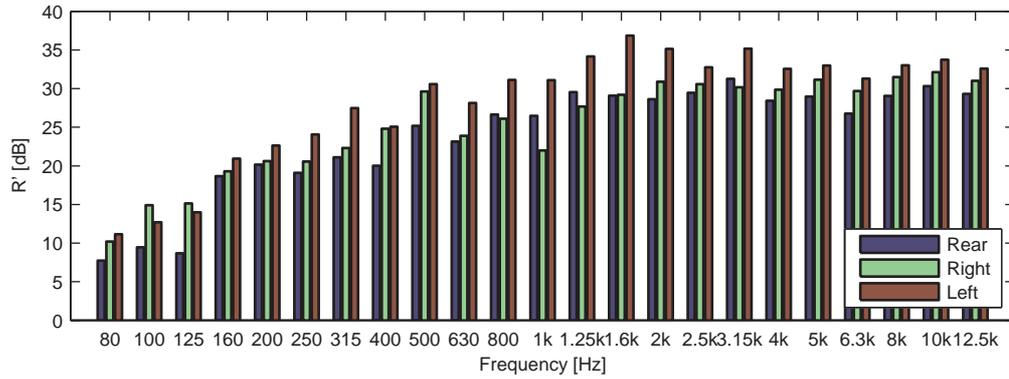
**Figure 3.6:** Calculated apparent sound reduction index  $R'$  for the three cabin facades represented in one-third octave bands.
