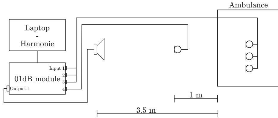
**Figure B.2:** Measurement setup for the airborne sound insulation measurement.
