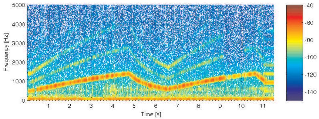
**Figure E.5:** Noise measured in the cabin where the ambulance is stationary and siren 1 turned on.
