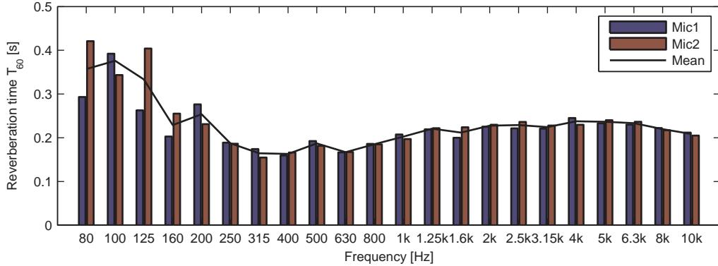
**Figure 3.1:** Results of the reverberation time measurement for the two microphones and the mean reverberation time measured in one-third octave bands.
