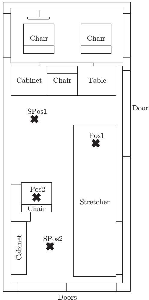
**Figure A.1:** Top view of the ambulance, with source and measurement positions marked by X.
