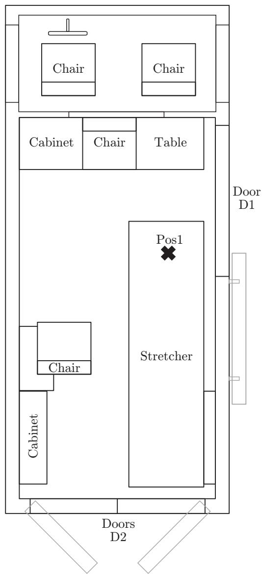
**Figure D.1:** Top view of the ambulance with the microphone position marked by **X**. Door D1 is a sliding door, and its opened position is sketched in gray. Door D2 is a two-part swinging door and its opened position is marked in gray.
