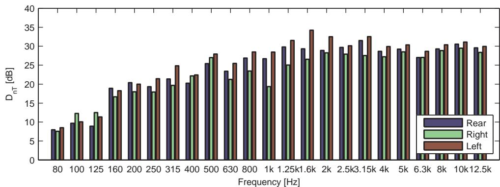
**Figure 3.5:** Calculated standardized level difference  $D_{nT}$  for the three cabin facades represented in one-third octave bands.
