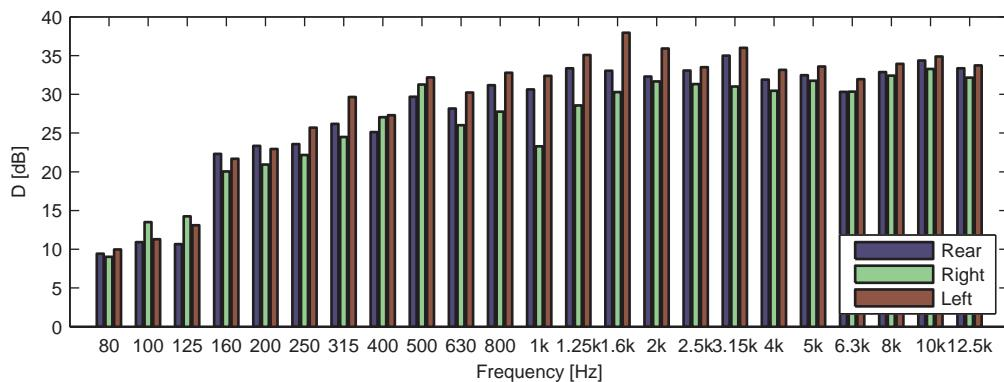
**Figure 3.4:** Calculated level difference  $D$  for the three cabin facades represented in one-third octave bands.
