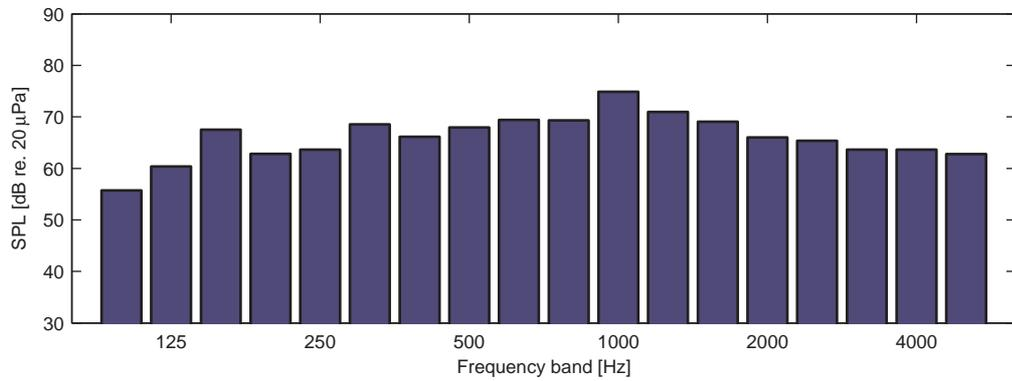
**Figure D.3:** Measured SPL in one-third octave bands from closing the side door of the ambulance.
