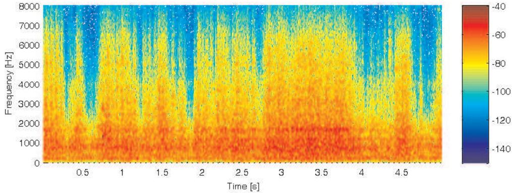
**Figure 3.16:** Spectrogram of the noise measured in the cabin when the ambulance is driving in the city with siren 2 turned on.
