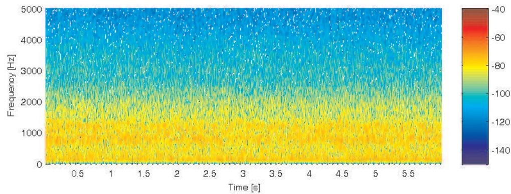
**Figure 3.18:** Spectrogram of the noise measured in the cabin when the ambulance is driving on the freeway with siren 2 turned on.
