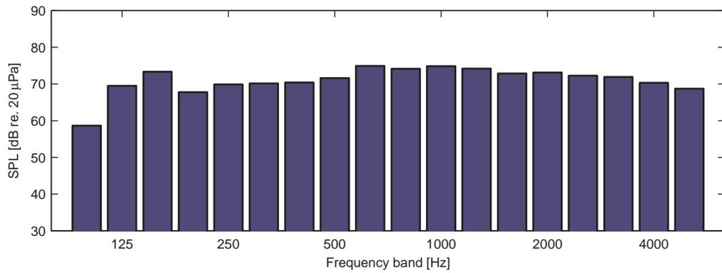
**Figure D.4:** Measured SPL in one-third octave bands from closing the rear left door of the ambulance.
