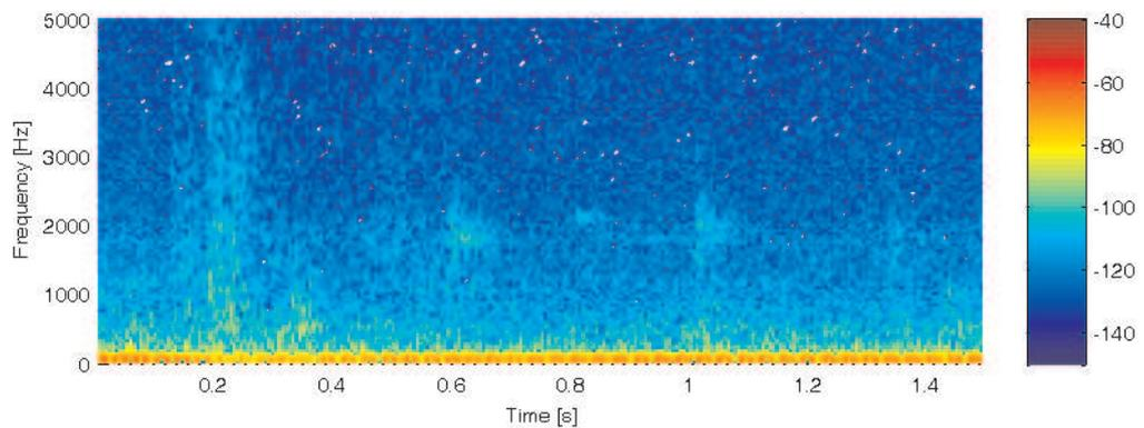
**Figure E.7:** Noise measured in the cabin where the ambulance is stationary.
