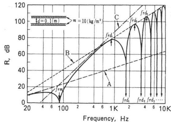
**Figure 4.3:** Frequency characteristics of double leaf wall transmission loss. [Maekawa and Lord, 1994, p. 179]
