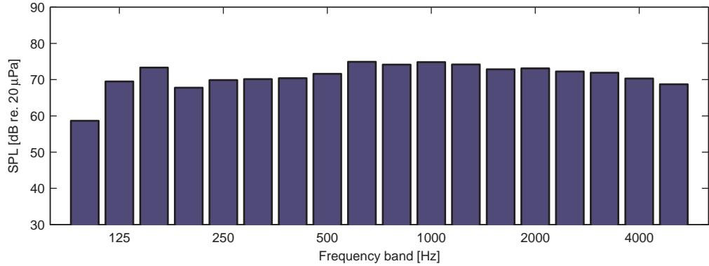
**Figure D.4:** Measured SPL in one-third octave bands from closing the rear left door of the ambulance.
