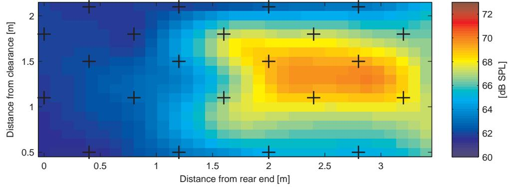
**Figure 3.8:** Right facade leakage, where + indicates a measurement point. Higher dB values means higher leakage and thus worse insulation at that point.
