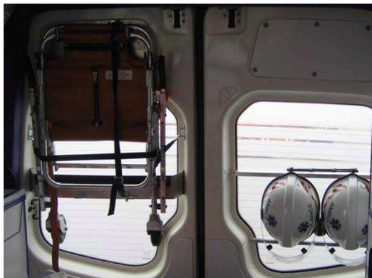
**Figure 4.4:** Picture of the helmets and the stretcher chair mounted inside the ambulance.
