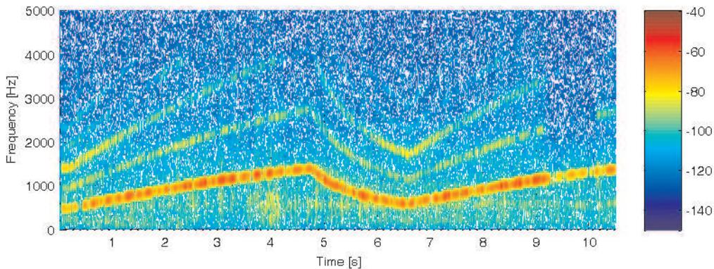
**Figure 3.12:** Spectrogram of the noise measured in the cabin when the ambulance is stationary and siren 1 is turned on. Note the duty cycle of siren 1 is seen.
