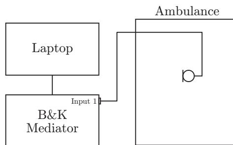
**Figure D.2:** Measurement setup for the closing door measurement.
