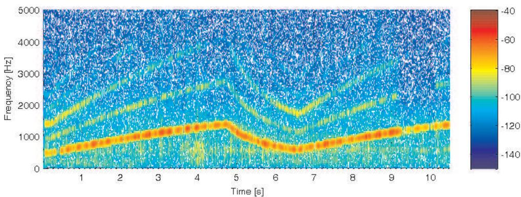
**Figure 3.12:** Spectrogram of the noise measured in the cabin when the ambulance is stationary and siren 1 is turned on. Note the duty cycle of siren 1 is seen.
