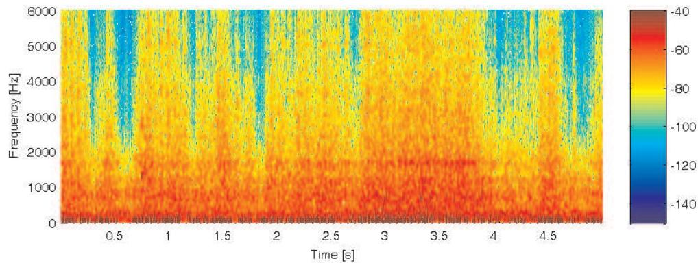
**Figure E.4:** Noise measured in the cabin when driving in the city with siren 2 on.
