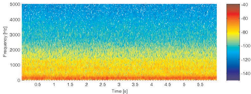
**Figure E.9:** Noise measured in the cabin when driving in on the freeway with siren 2 on.
