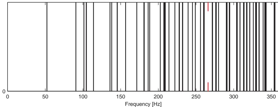
**Figure 3.3:** Room modes in the cabin below 360 Hz, where the calculated Schroeder frequency is marked by the red lines at 266 Hz.
