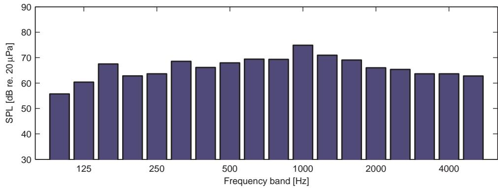
**Figure D.3:** Measured SPL in one-third octave bands from closing the side door of the ambulance.
