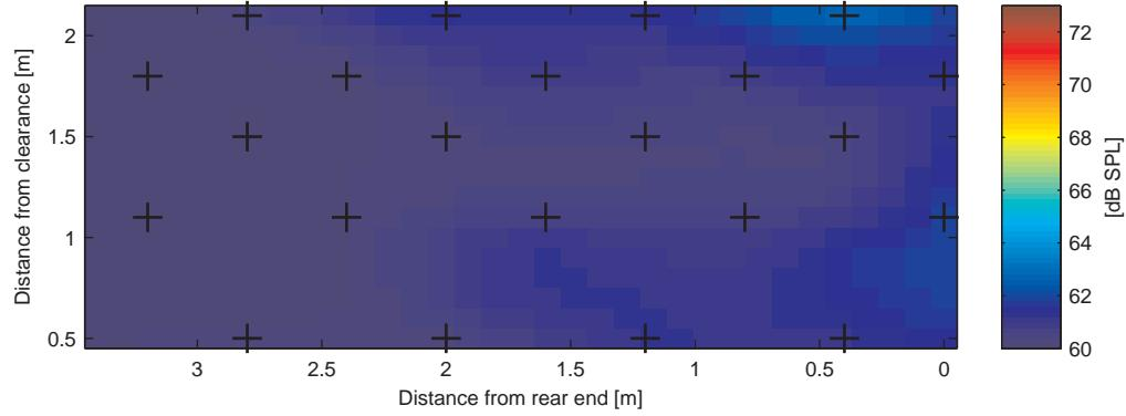
**Figure 3.7:** Left facade leakage, where + indicates a measurement point. Higher dB values means higher leakage and thus worse insulation at that point.
