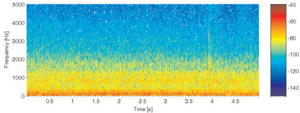
**Figure E.13:** Noise measured in the cabin when driving on highway with the siren turned off.
