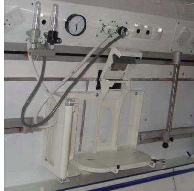
**Figure 4.5:** Picture of the defibrillator mounting.
