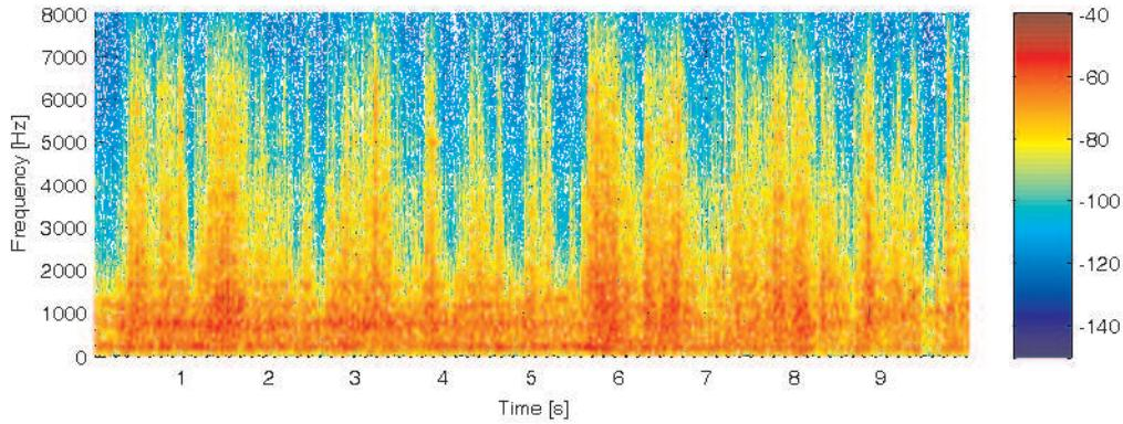
**Figure 3.15:** Spectrogram of the noise measured in the cabin when the ambulance is driving in the city with siren 1 turned on.
