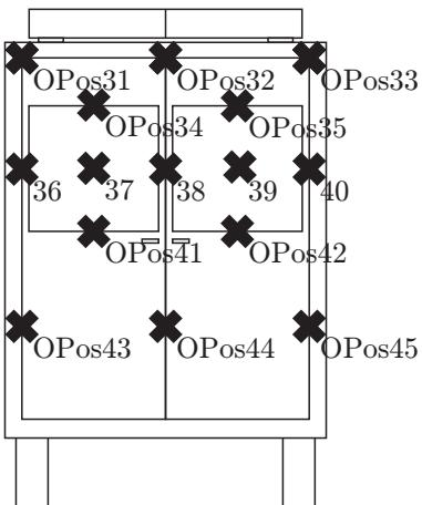
**Figure C.3:** Measurement positions for the facade leakage measurement for the rear end.
