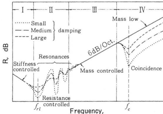
**Figure 4.2:** Frequency characteristics of single wall transmission loss. [Maekawa and Lord, 1994, p. 173]
