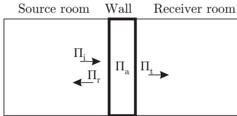
**Figure 4.1:** Illustration of sound transmission through a wall.
