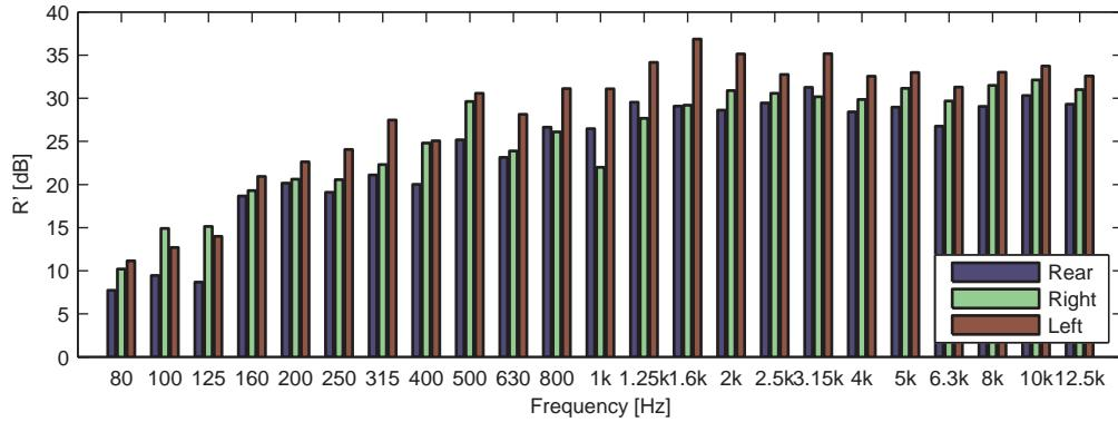
**Figure 3.6:** Calculated apparent sound reduction index  $R'$  for the three cabin facades represented in one-third octave bands.
