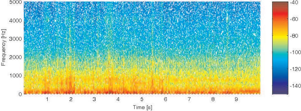
**Figure E.10:** Noise measured in the cabin when driving on freeway with the siren turned off.
