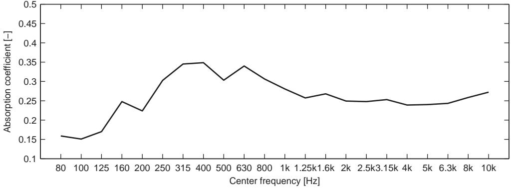
**Figure 3.2:** Absorption coefficient for the mean reverberation time in one-third octave bands.
