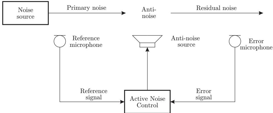
**Figure 4.7:** Principle of a feedforward active noise control system.
