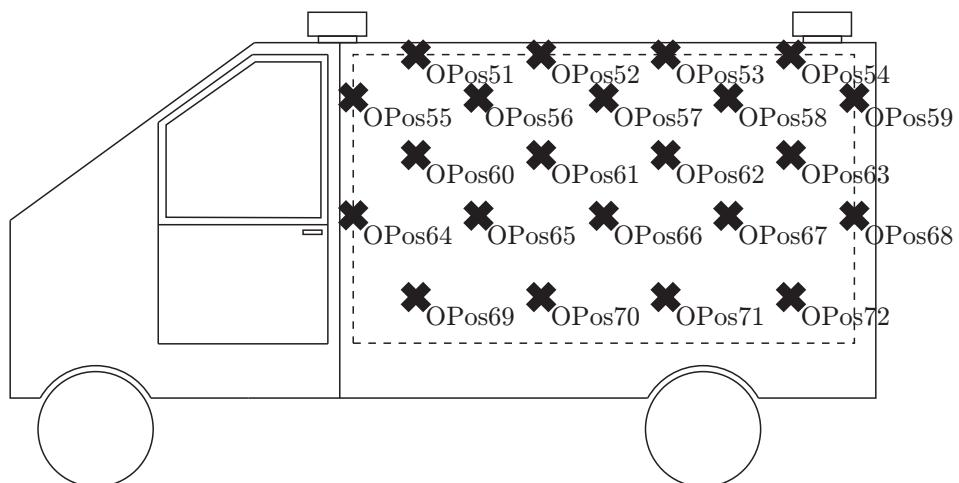
**Figure C.2:** Measurement positions for the facade leakage measurement for the left side of the ambulance.
