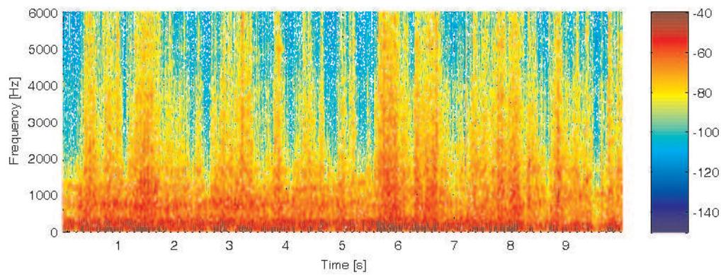
**Figure E.3:** Noise measured in the cabin when driving in the city with siren 1 on.
