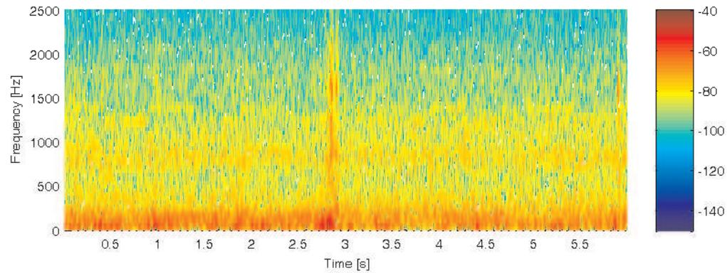
**Figure E.12:** Noise measured in the cabin when driving on highway with siren 2 turned on.
