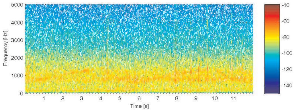
**Figure 3.17:** Spectrogram of the noise measured in the cabin when the ambulance is driving on the freeway with siren 1 turned on.
