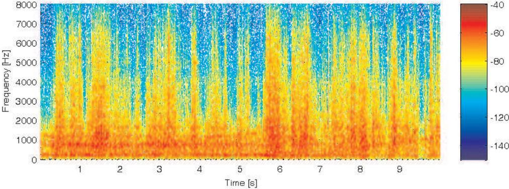
**Figure 3.15:** Spectrogram of the noise measured in the cabin when the ambulance is driving in the city with siren 1 turned on.
