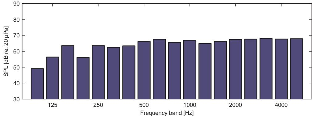
**Figure D.5:** Measured SPL in one-third octave bands from closing the rear right door of the ambulance.
