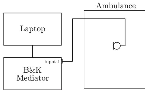
**Figure E.2:** Measurement setup for noise exposure measurement.
