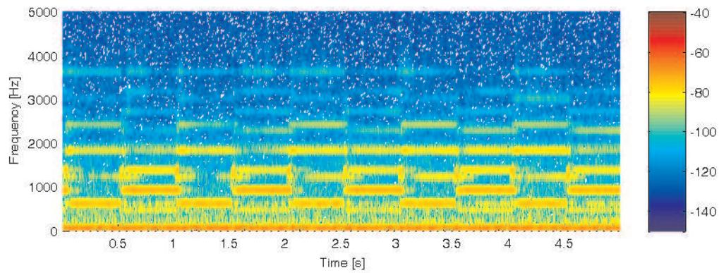
**Figure E.6:** Noise measured in the cabin where the ambulance is stationary and siren 2 turned on.
