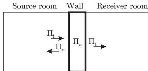
**Figure 4.1:** Illustration of sound transmission through a wall.
