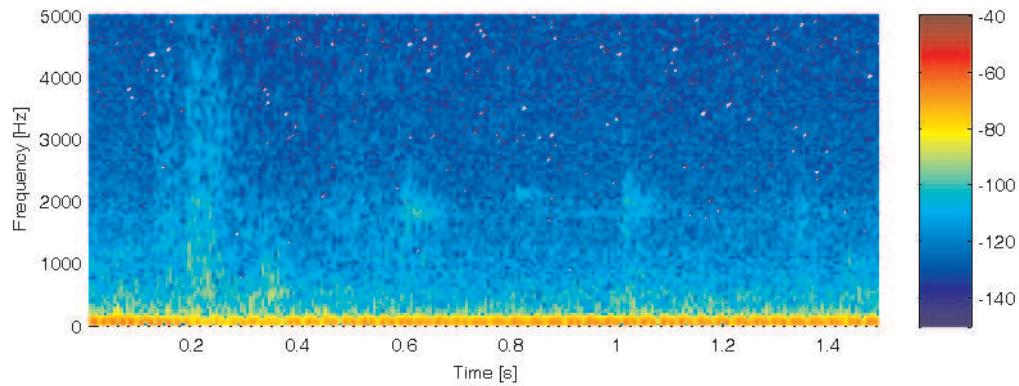
**Figure E.7:** Noise measured in the cabin where the ambulance is stationary.
