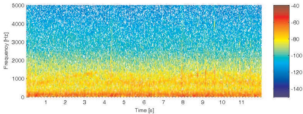
**Figure E.8:** Noise measured in the cabin when driving in on the freeway with siren 1 on.
