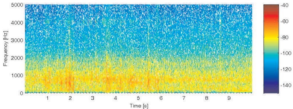
**Figure 3.19:** Spectrogram of the noise measured in the cabin when the ambulance is driving on the freeway with the siren turned off.
