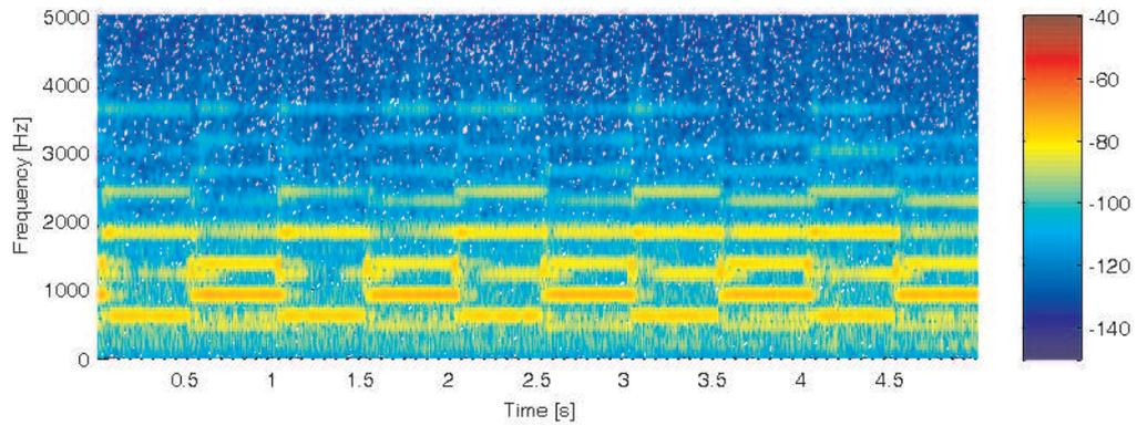
**Figure 3.13:** Spectrogram of the noise measured in the cabin when the ambulance is stationary and siren 2 is turned on. Note the duty cycle of siren 2 is seen.
