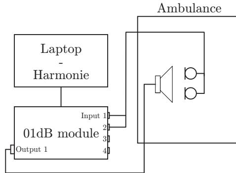
**Figure A.2:** Measurement setup for the reverberation time measurement.
