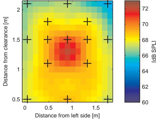
**Figure 3.9:** Rear facade leakage, where + indicates a measurement point. Higher dB values means higher leakage and thus worse insulation at that point.
