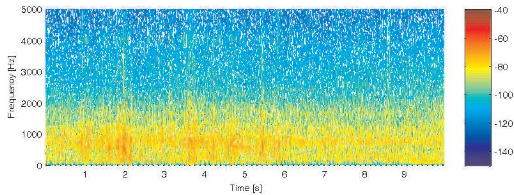
**Figure 3.19:** Spectrogram of the noise measured in the cabin when the ambulance is driving on the freeway with the siren turned off.
