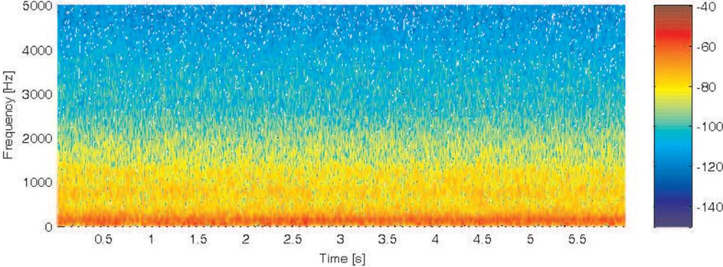
**Figure E.9:** Noise measured in the cabin when driving in on the freeway with siren 2 on.
