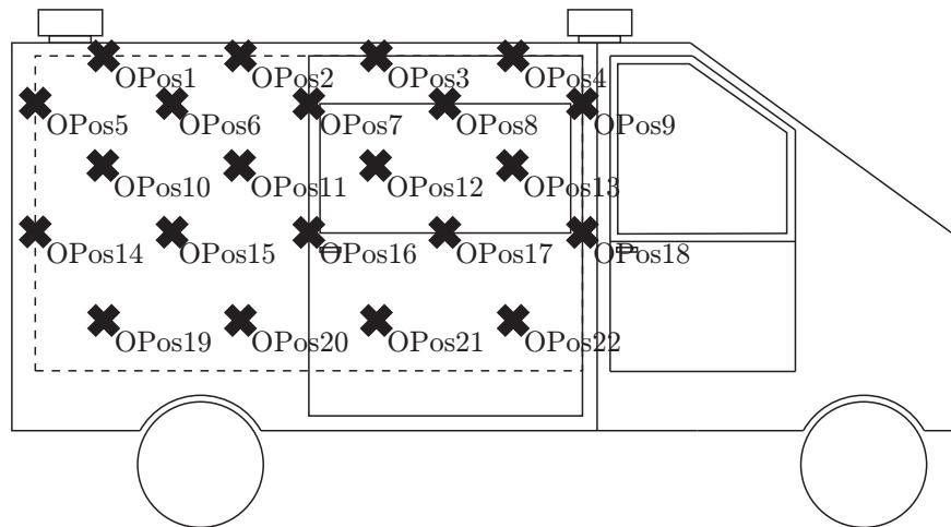
**Figure C.1:** Measurement positions for the facade leakage measurement for the right side of the ambulance.
