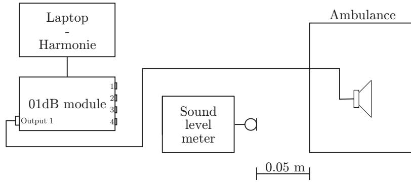
**Figure C.4:** Measurement setup for the facade leakage measurement.
