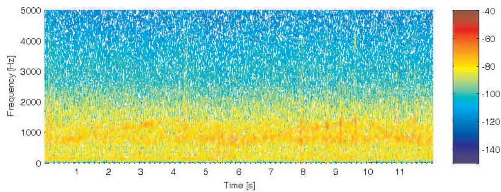
**Figure 3.17:** Spectrogram of the noise measured in the cabin when the ambulance is driving on the freeway with siren 1 turned on.
