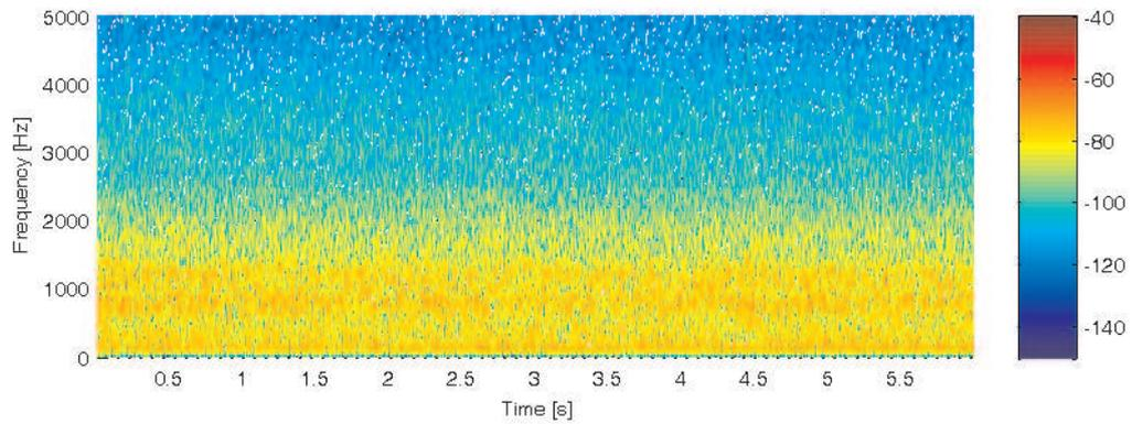
**Figure 3.18:** Spectrogram of the noise measured in the cabin when the ambulance is driving on the freeway with siren 2 turned on.
