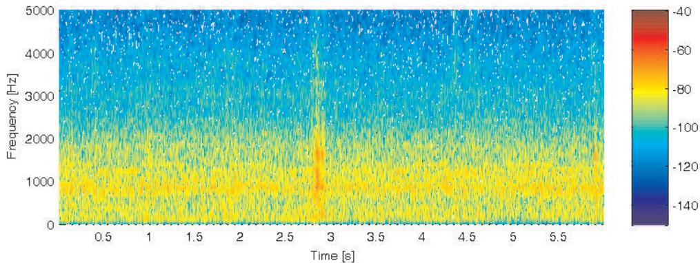
**Figure 3.21:** Spectrogram of the noise measured in the cabin when the ambulance is driving on the highway with siren 2 turned on.
