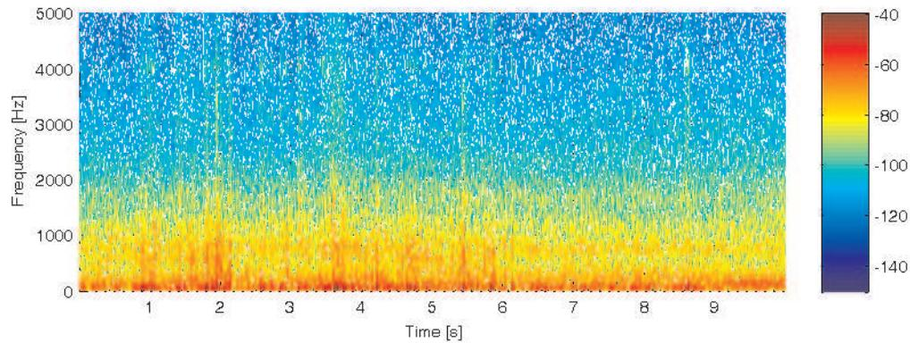
**Figure E.10:** Noise measured in the cabin when driving on freeway with the siren turned off.
