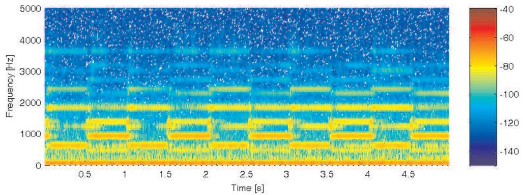
**Figure E.6:** Noise measured in the cabin where the ambulance is stationary and siren 2 turned on.
