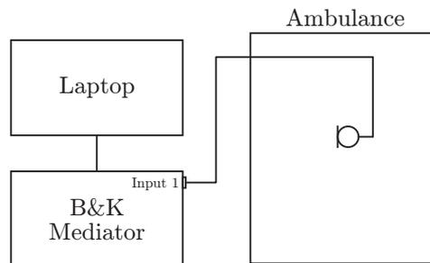
**Figure D.2:** Measurement setup for the closing door measurement.
