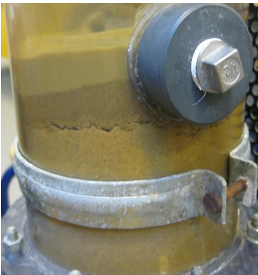
Figure 123 Crack between filter cake and formation
