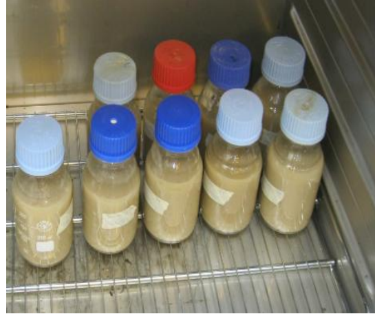
Figure 57 Aging samples in the oven at 74 deg. C
