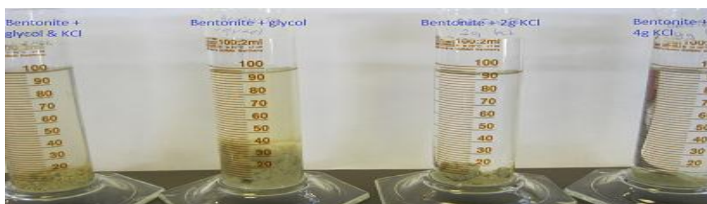
Figure 25 Inhibitive Swell Test Set up for Bentonite sample
