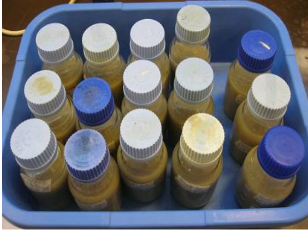
Figure 56 Aging mud samples at ambient temperature.
