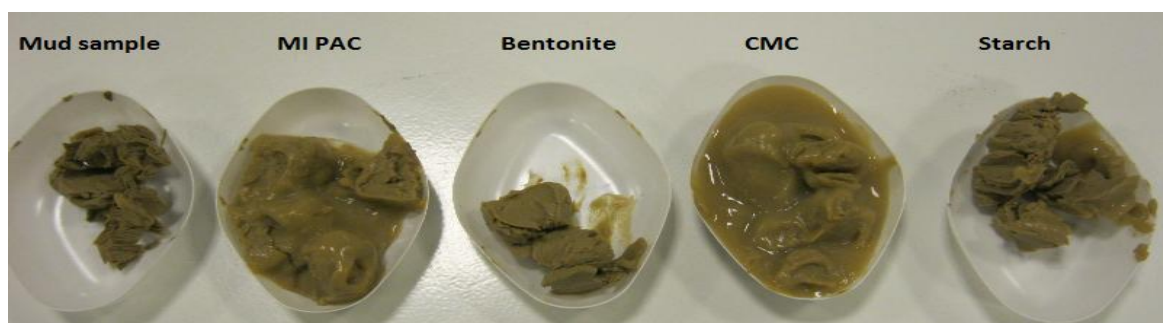
Figure 35 Filter cakes formed using different additives and sea water source.
