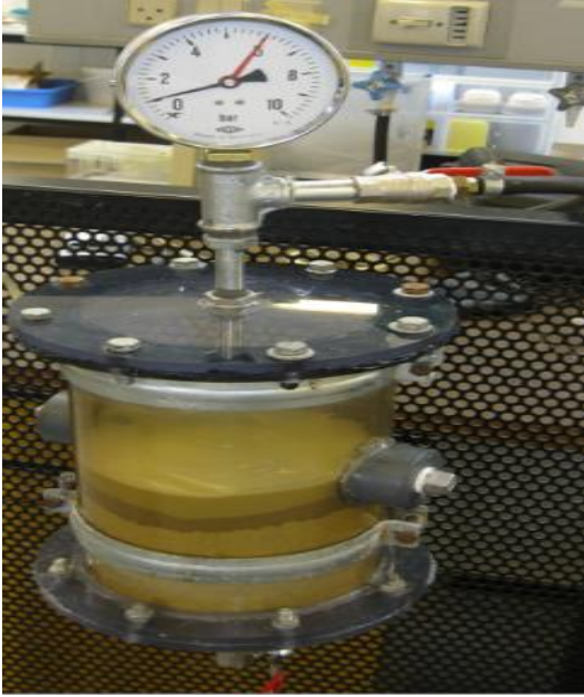
Figure 121 Formation of thicker layer of filter cake.
