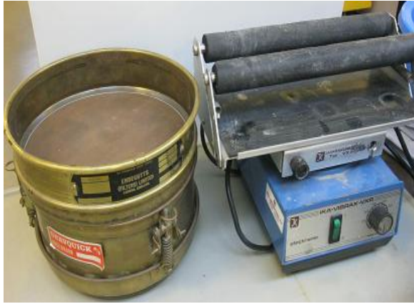
Figure 27 Sand content test apparatus.
