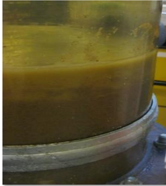
Figure 126 Section showing mud and formation layers.
