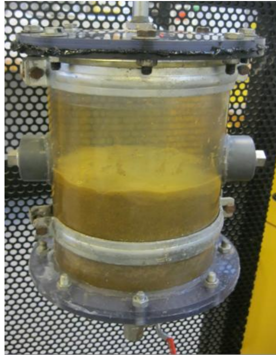
Figure 128 Section showing reduced mud layer.
