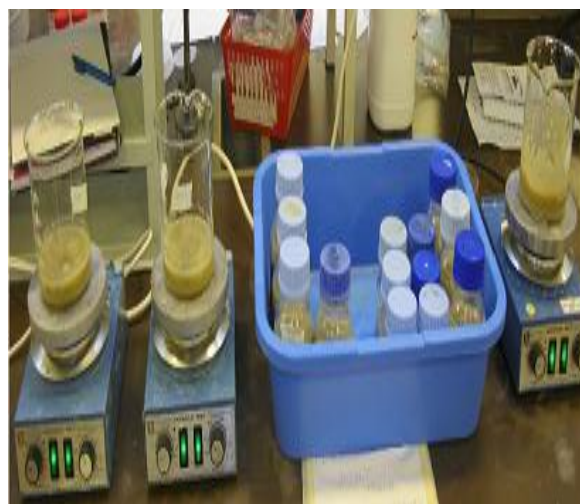
Figure 32 Agitation and heating of mud samples.
