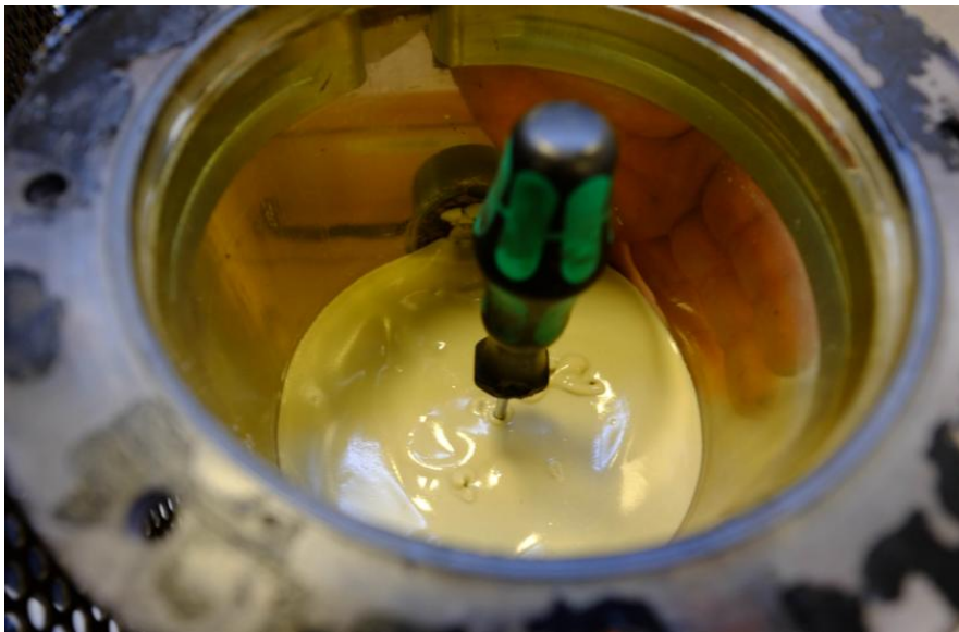
Figure 129 Ascertaining filter cake development on the wet sand formation by poking with a hard metallic object.
