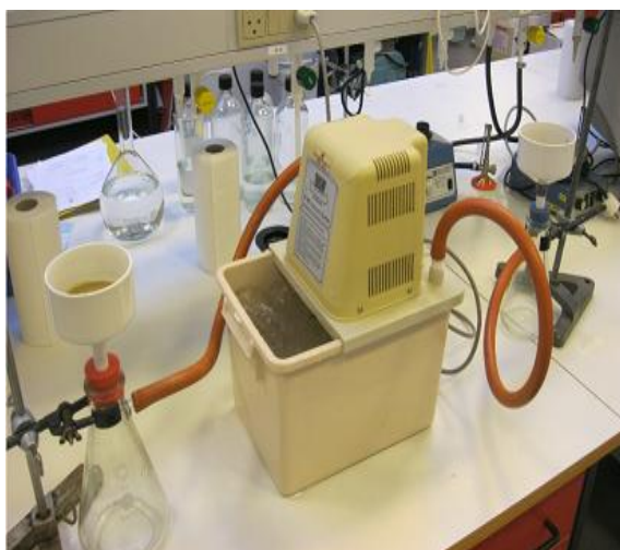
Figure 31 Filtration set up using water vacuum system.
