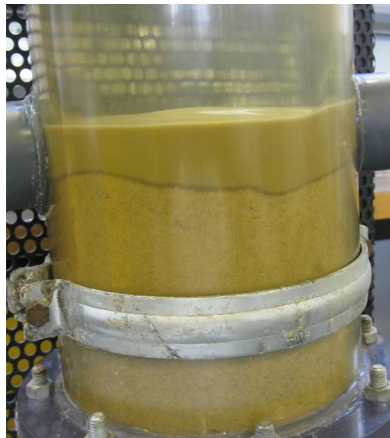
Figure 120 Section showing thin filter cake layer.
