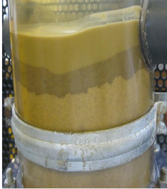
Figure 122 Section showing thicker filter cake layer.
