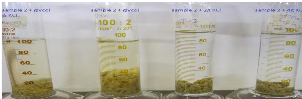
Figure 21 Inhibitive Swell Test Set up for mud sample 2
