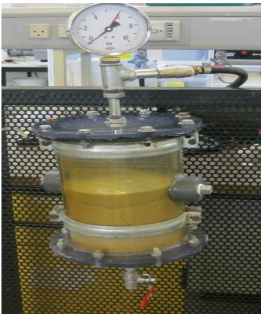
Figure 119 Formation of thin layer of filter cake.
