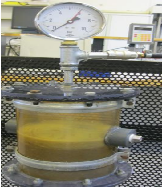
Figure 125 Set up with wet sand formation.
