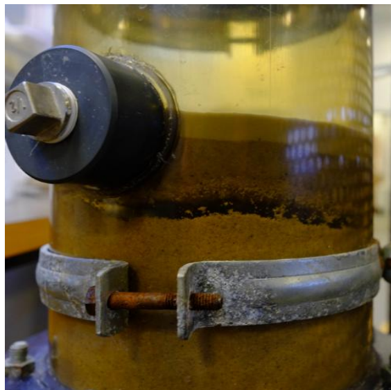
Figure 124 Expansion of crack due to pressure.
