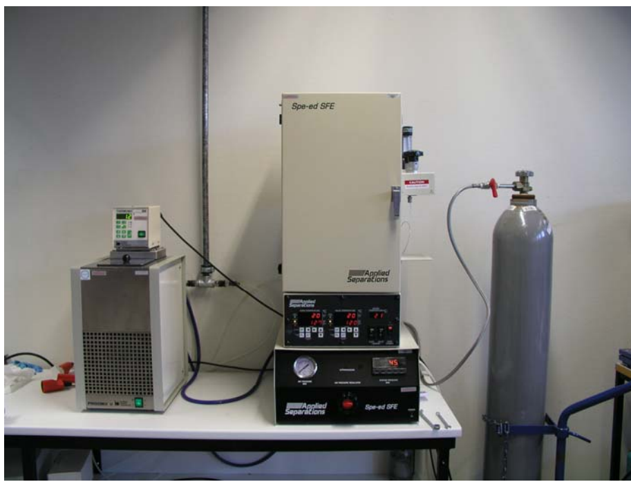
Figure 23: Supercritical CO 2 Equipment
