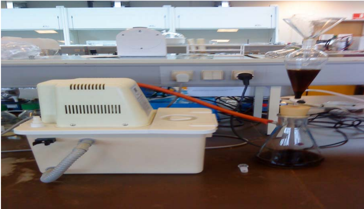
Figure 20: Saturation setup for chalk core sample
