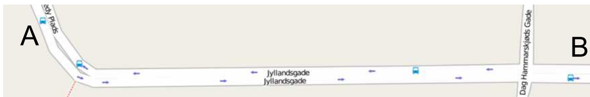
Figure 58 Error introduced by the absence of the bus stop arrival time at a bus stop
