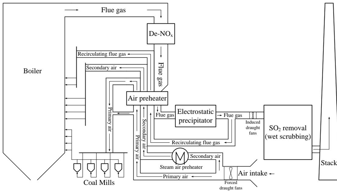
**Figure 3.4:** Flow diagram of the channels where the flue gas and air are led before and after the air preheater.
