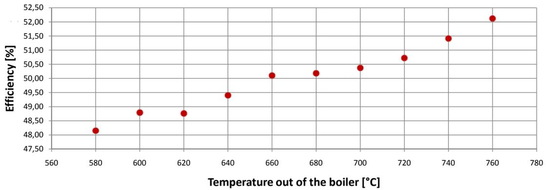
**Figure 7.1:** Efficiency as a function of temperature from the boiler and pressure from the feedwater pumps.
