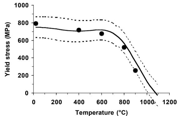
**Figure 2.1:** Evolution of yield stress as a function of temperature: solid circles indicate measurements; solid line indicates mean Gaussian processes predictions; broken lines indicate predicted error bounds.[Tancret and Bhadeshia 2003]
