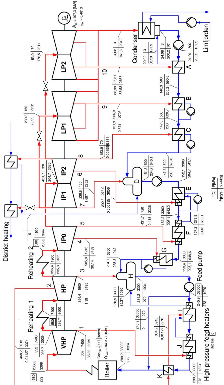
Figure 6.1: Key numbers in the water/steam cycle from the model when simulating NJV3 at full load.
