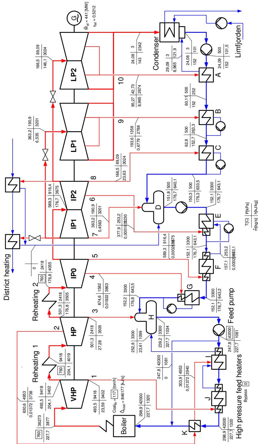
Figure 7.2: Key numbers in the water/steam cycle from the model when simulating 769 °C from the boiler and 42 MPa from the high pressure feedwater pump.
