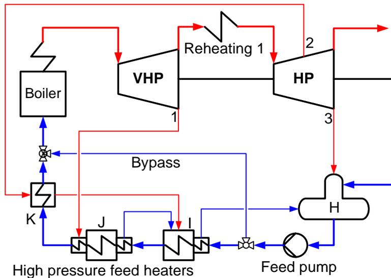
Figure 5.6: Bypass over the last three feedwater heat exchangers.
