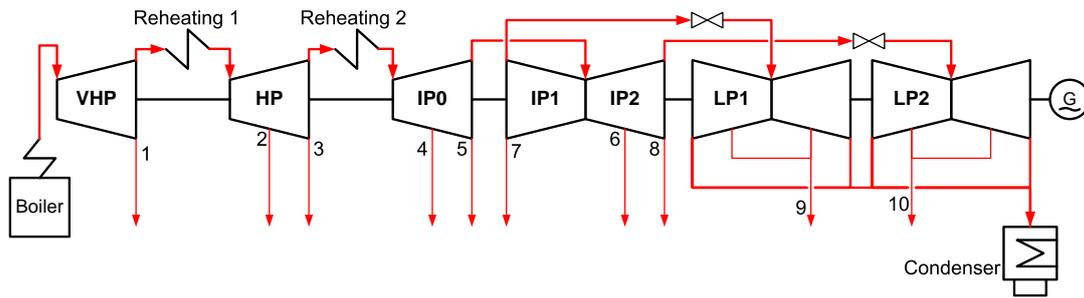
Figure 5.4: Diagram over the turbine and its steam outlets.
