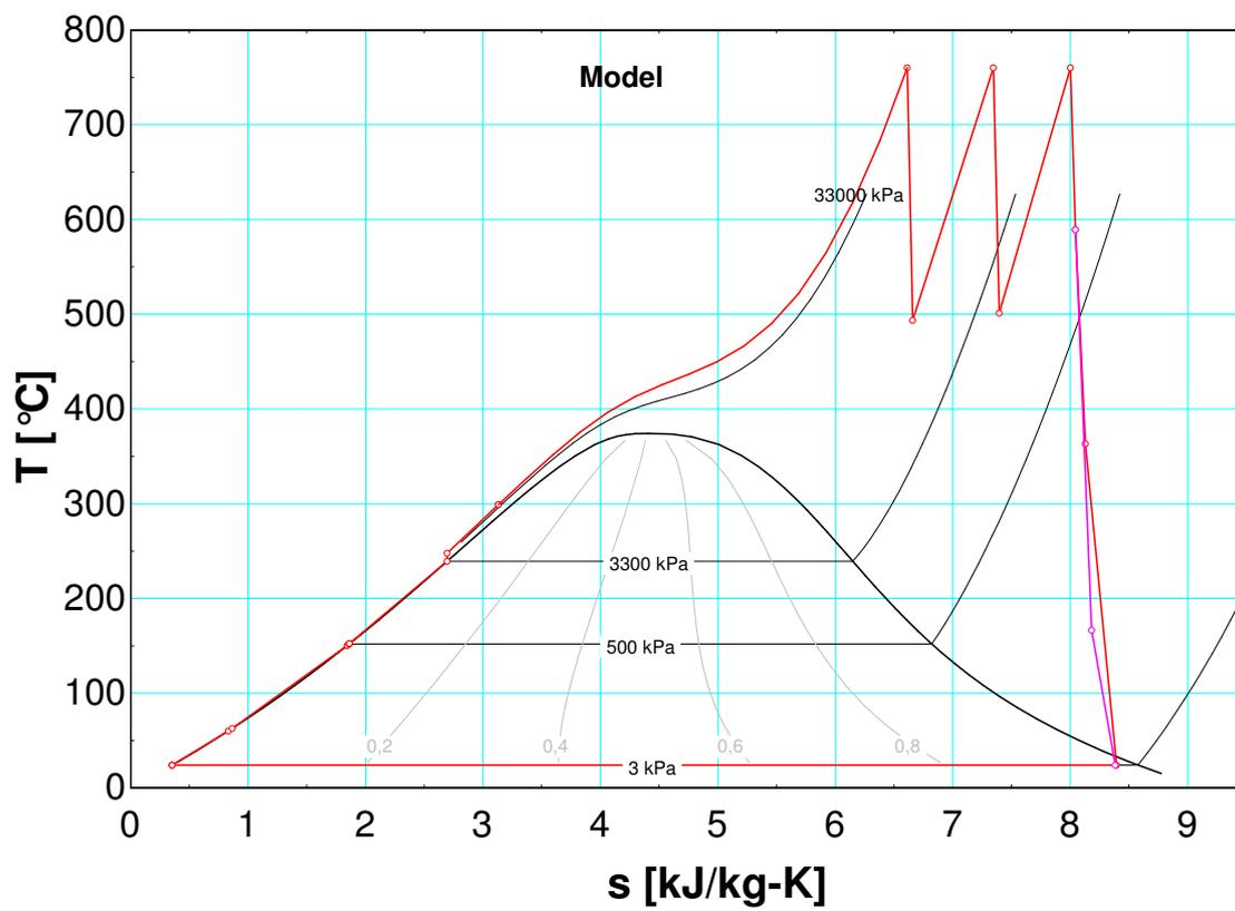
**Figure 7.3:** *T-s diagram over the water/steam cycle when simulating 769 °C from the boiler and 42 MPa from the high pressure feedwater pump.*
