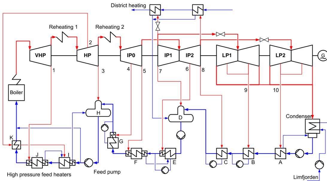
**Figure 3.2:** A representation of the water/steam cycle in Unit 3 in Nordjyllandsværket.
