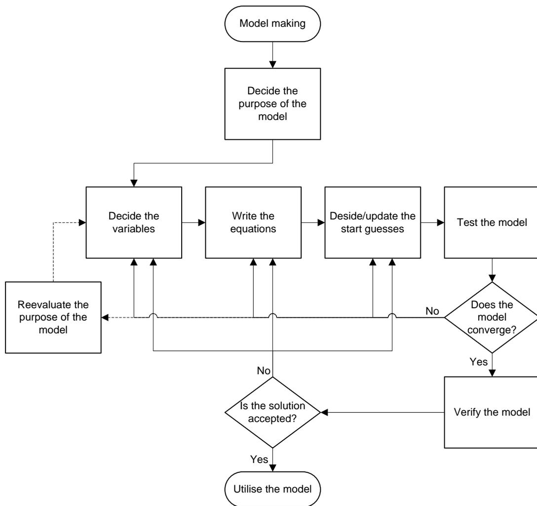
**Figure 4.1:** Flowchart that shows the process of building the model in EES.
