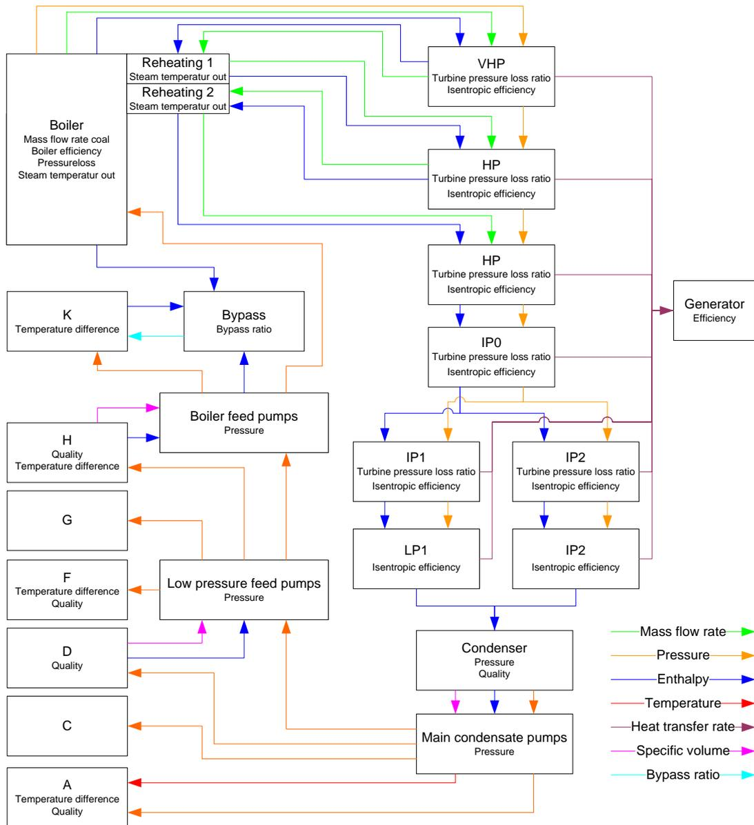
**Figure 5.3:** Diagram that shows how the modules in the model are connected. Under the name of the module are listed those variables that are input to the model.
