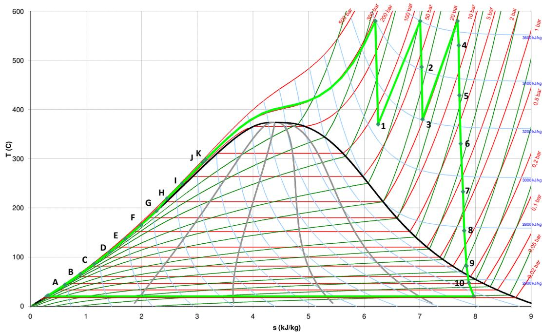
Figure 3.3: A T-s diagram over the water/steam cycle in Unit 3 in Nordjyllandsværket.
