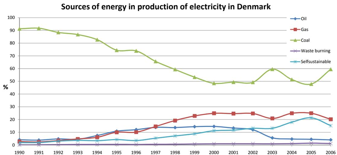
**Figure 1.1:** Overview over the main sources of energy in production of electricity in Denmark. [Dal and Zarnaghi 2007]
