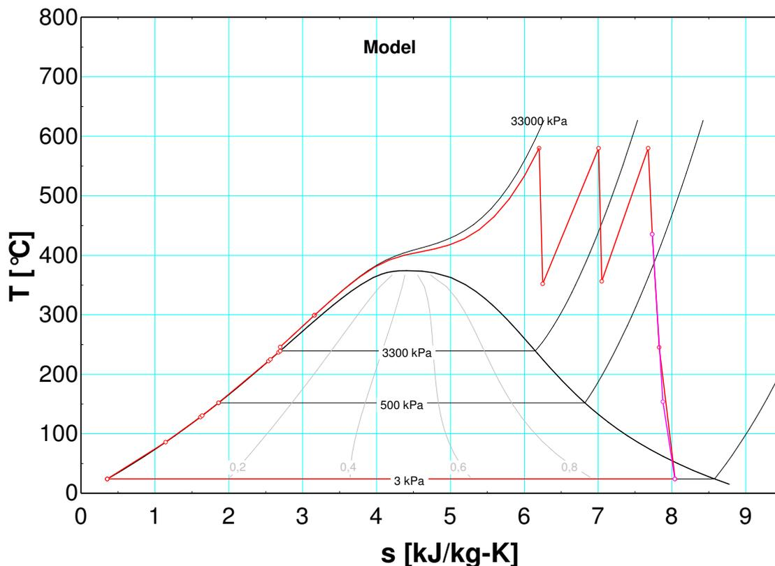
**Figure 6.2:** T-s diagram over the water/steam cycle when simulating NJV3 at full load.
