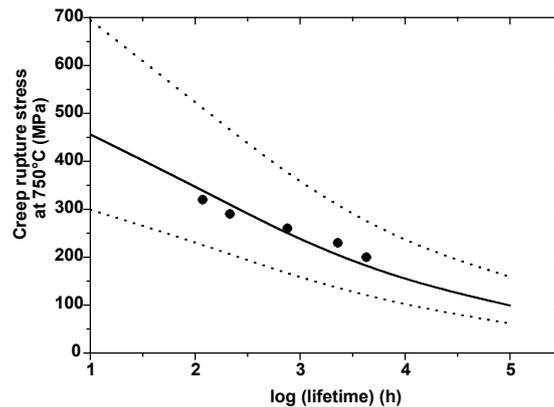
**Figure 2.2:** Creep rupture stress as a function of lifetime. Circles: measurements; solid line: mean Gaussian processes predictions; dotted lines: predicted error bounds. [Tancret et al. 2003]
