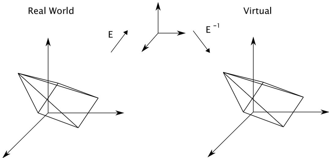
**Figure 5.2:** *The position and rotation of a light probe can be restored in the virtual scene using a reference frame.*
