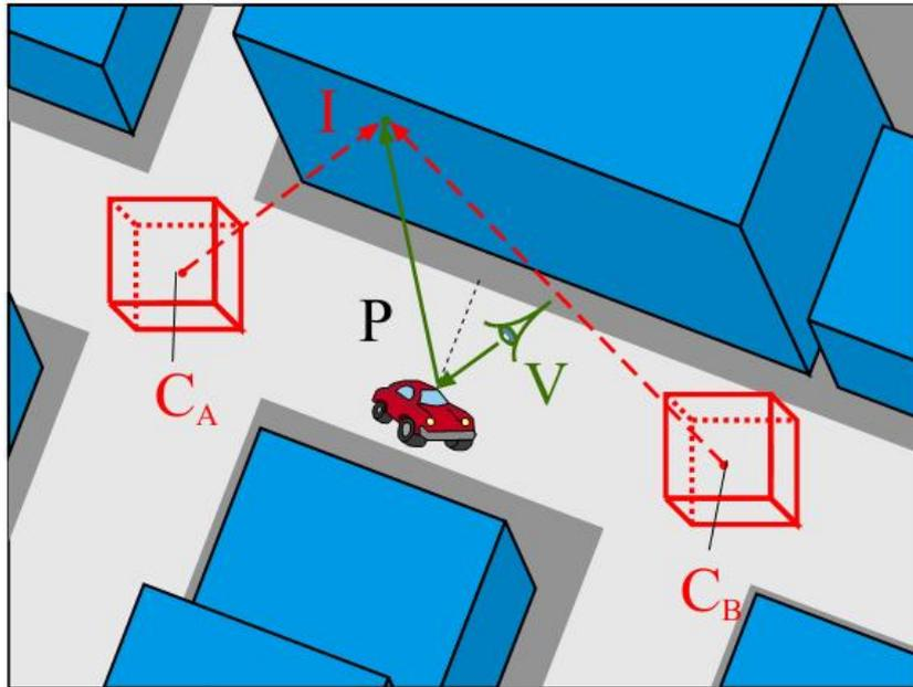
**Figure 2.1:** Reference Environment Maps ( $C_A$  and  $C_B$ ) are prerendered at representative locations in the scene. The local reflection at point  $P$  may then be calculated based on the intersection point  $I$  and the maps  $C_A$ ,  $C_B$ . From [ML03].
