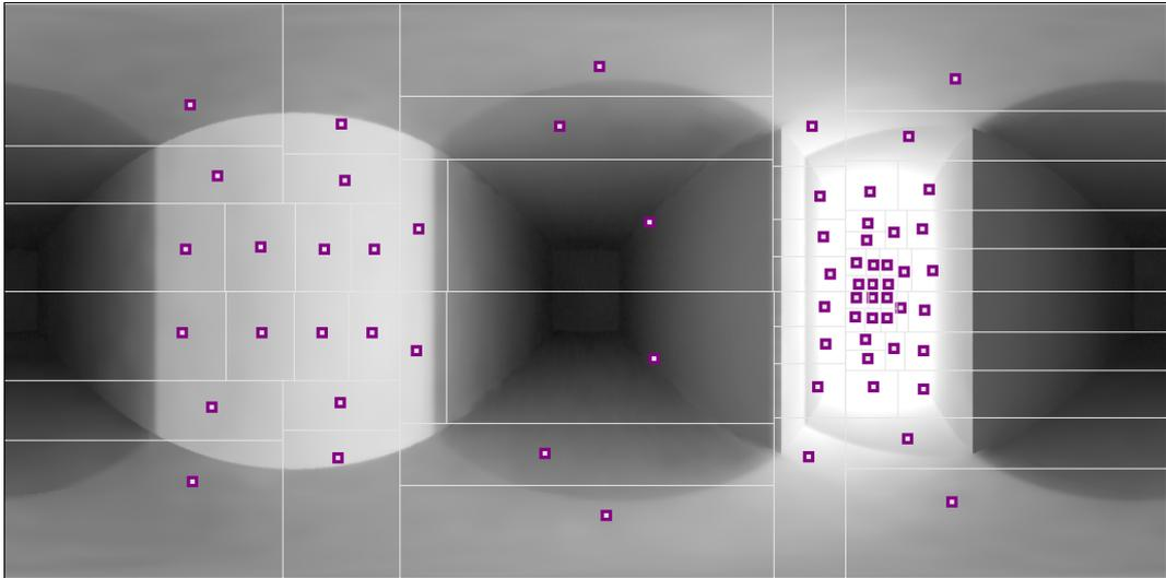
**Figure 4.6:** *Result of applying the Median Cut algorithm to the LL map. The purple squares indicate the positions of where the directional light should be placed to approximate the incident radiance.*
