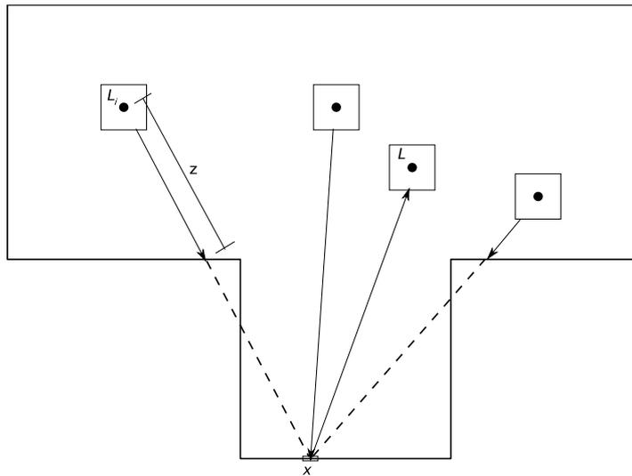
**Figure 5.5:** A light probe is not valid if the distance from a surface point  $x$  to the position of the light probe is bigger than the  $Z$  value stored in the light probe for the same direction.
