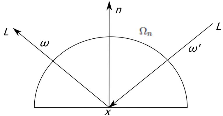
**Figure 5.3:** Visualisation in 2-D of the terms in Equation 5.2 where  $L$  is the exitant radiance and  $L'$  is the incident radiance. The direction vectors  $\omega$  and  $\omega'$  are unit-length,  $\Omega_n$  is the hemisphere defined on a surface point  $x$  with the normal  $n$ .
