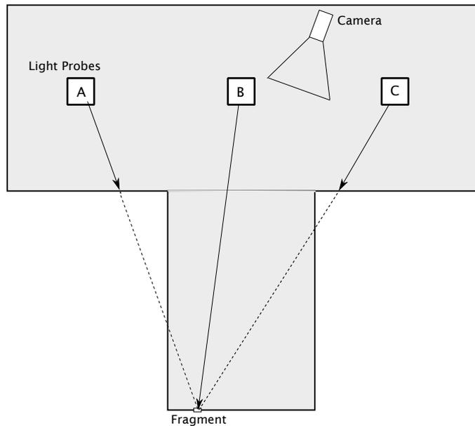
**Figure 4.4:** *The distance from a fragment to the light probes is calculated and compared to distances stored in each light probe. If the distance from fragment to light probe is smaller than the stored value the light probe is not visible and is omitted when calculating the exitant radiance from the fragment.*
