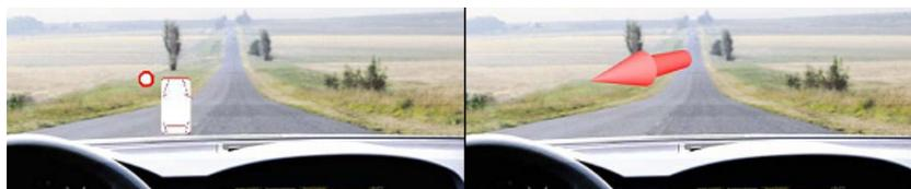
**Figure 1.1:** AR used in cars to improve security by visualising areas that require the drivers attention. (Adopted from [TSK<sup>+</sup>05].)
