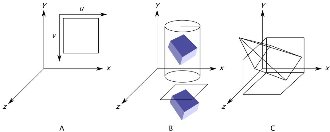
**Figure 5.1:** *Different types of mapping texture to geometry. In A is shown  $uv$ -mapping, B exemplifies analytical mappings such as cylindrical and planar projection, and in C is shown projection from an arbitrary view point.*
