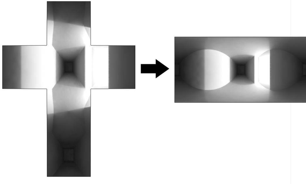
**Figure 4.5:** *The incoming radiance at the position of the object along with the distance to the scene geometry is sampled and stored in a cube map. The cube map is then converted to LL map on the GPU.*
