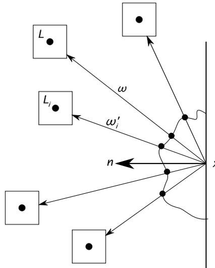
**Figure 5.4:** The pixel value stored in a light probe  $L_i(\omega_i')$  is a sampling of the radiance distribution at point  $x$ . To generate a dynamic EM at some position in the scene the value of  $L(x, \omega)$  must be determined.
