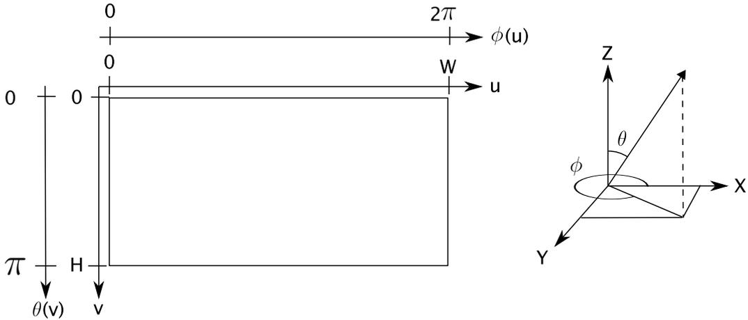
Figure 5.7: Mapping from spherical coordinates to LL map.
