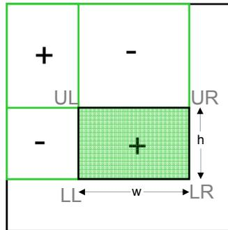
Figure 6.2: Summation using a SAT. Adapted from [HS05].
