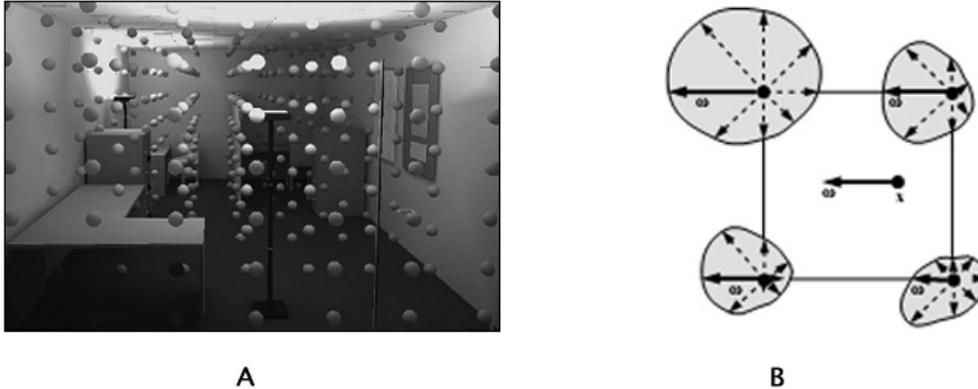
**Figure 2.2:** *Figure A shows a scene rendered using an Irradiance Volume with each cell represented with a sphere. Figure B illustrates how to calculate the irradiance for a vertex by interpolating between the nearest cells. From [GSHG98].*
