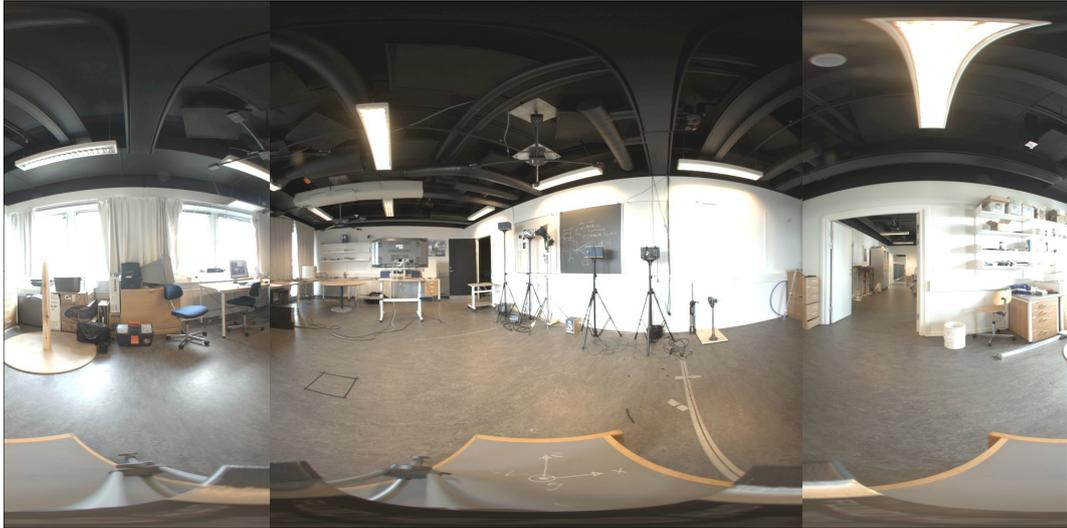
**Figure 4.1:** *Example of a light probe in Latitude-Longitude format. The light probe is created by stitching two photos taken with a fish-eye lens. The light probe is captured in HDR so the pixel values have here been mapped to a low-dynamic range to better visualise them. (Courtesy of Claus B. Madsen)*
