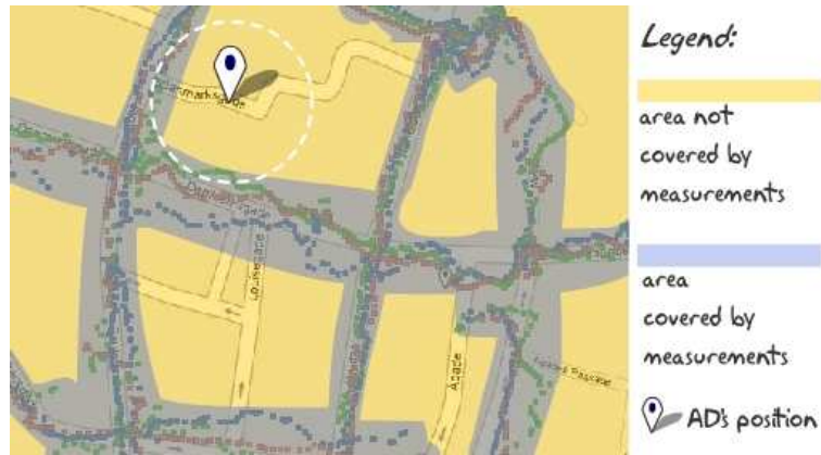
Figure C.3: The AD's position is included in the area not covered by measurements
