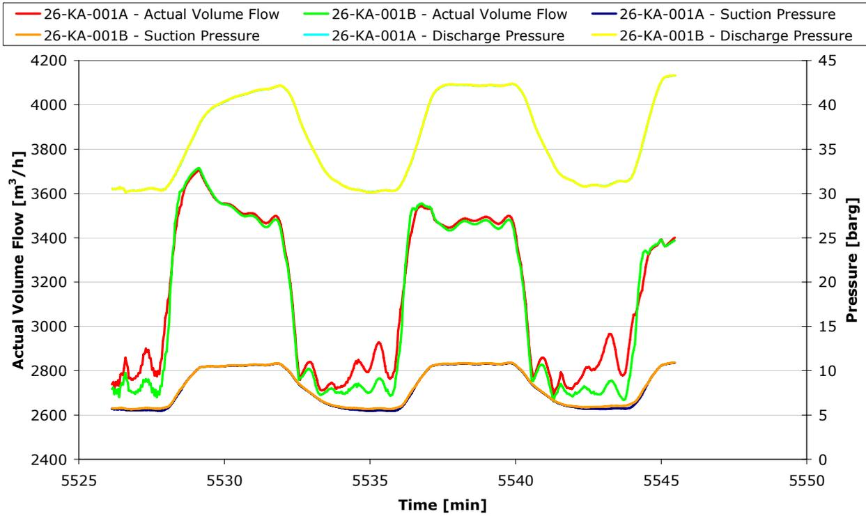
Figure 5.48. Actual volume flow, suction and discharge pressures for 1<sup>st</sup> section compressors. Slug amplitude 70 % of normal flow and slug period 8 minutes.
