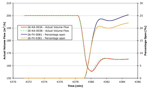
**Figure 4.28. Anti-surge control activation on 3<sup>rd</sup> section compressors upon an inlet gas flow reduction to 50 % of normal flow.  $K_c=0.5$ ,  $T_i=0.15$  min, and  $T_d=0$ .**
