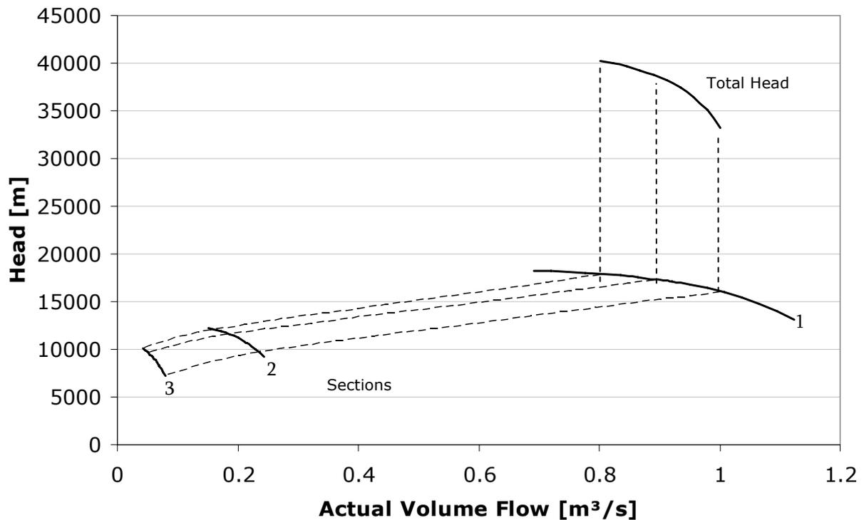
**Figure 2.17. Polytopic head curves for the three serial connected compressors on the OGPU and the resulting total polytopic head curve.**
