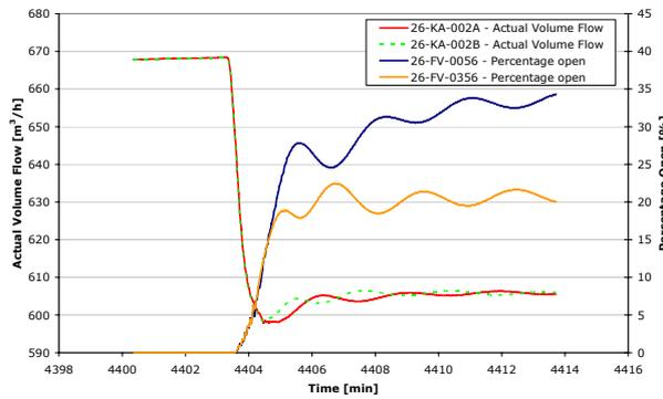
**Figure 4.30. Anti-surge control activation on 2<sup>nd</sup> section compressors upon an inlet gas flow reduction to 50 % of normal flow.  $K_c=4$ ,  $T_i=0.2$  min, and  $T_d=0$ . Max. overshoot 13 %.**
