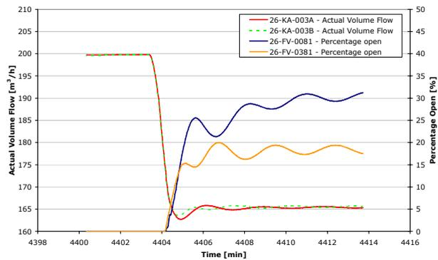
**Figure 4.31. Anti-surge control activation on 3<sup>rd</sup> section compressors upon an inlet gas flow reduction to 50 % of normal flow.  $K_c=4$ ,  $T_i=0.2$  min, and  $T_d=0$ . Max. overshoot 15 %.**
