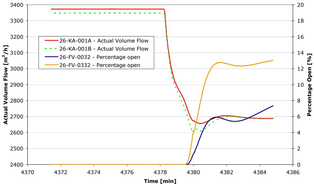
**Figure 4.26. Anti-surge control activation on 1<sup>st</sup> section compressors upon an inlet gas flow reduction to 50 % of normal flow.  $K_c=0.5$ ,  $T_i=0.15$  min, and  $T_d=0$ .**
