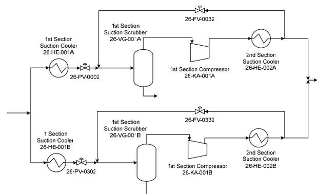
Figure 5.36. Alternative configuration of suction throttling valves.
