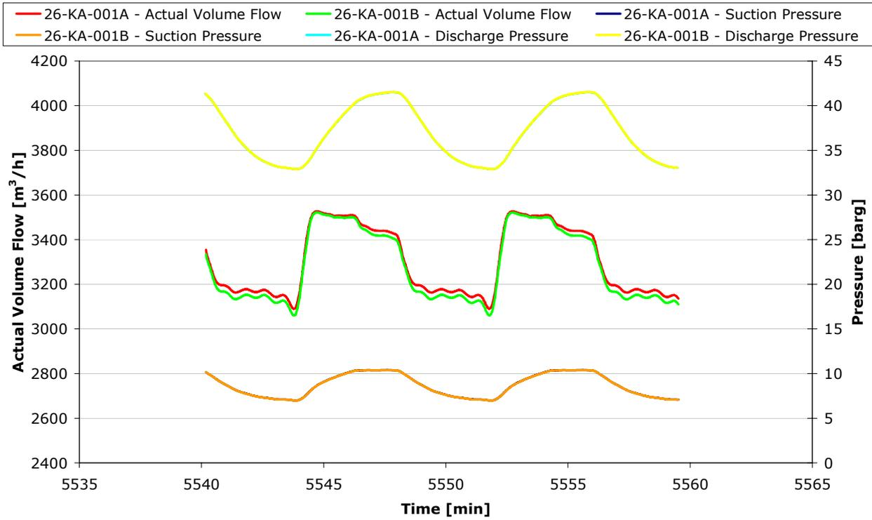
Figure 5.42. Actual volume flow, suction and discharge pressures for 1<sup>st</sup> section compressors. Slug amplitude 30 % of normal flow and slug period 8 minutes.
