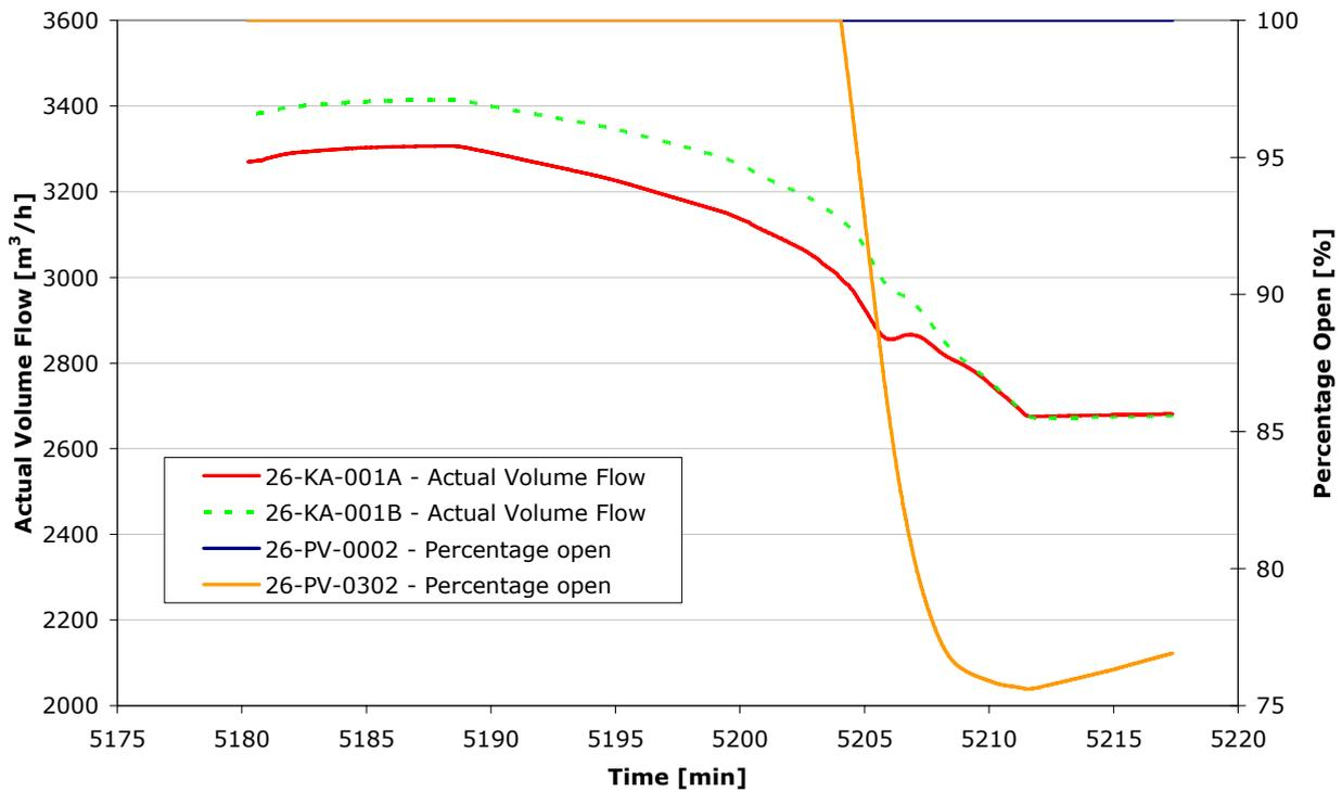
**Figure 4.33. Effect of load-sharing control on 1<sup>st</sup> section compressors. The load share is enabled at approximately 3000 m<sup>3</sup>/h.**
