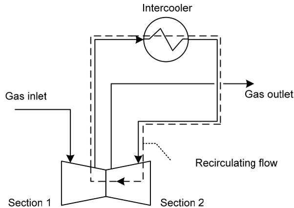
**Figure 2.8. Back-to-back compressor arrangement.**
