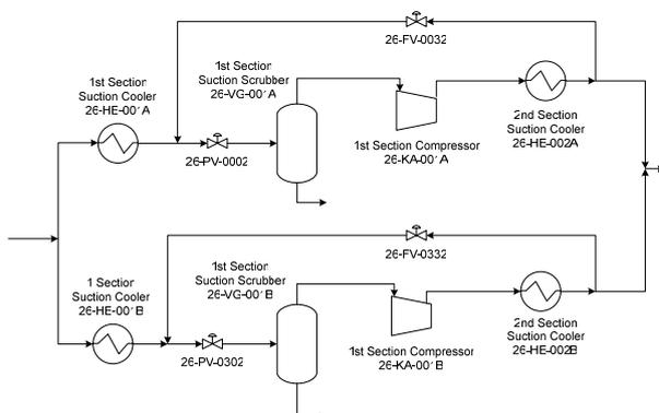
Figure 5.35. Current configuration of suction throttling valves.
