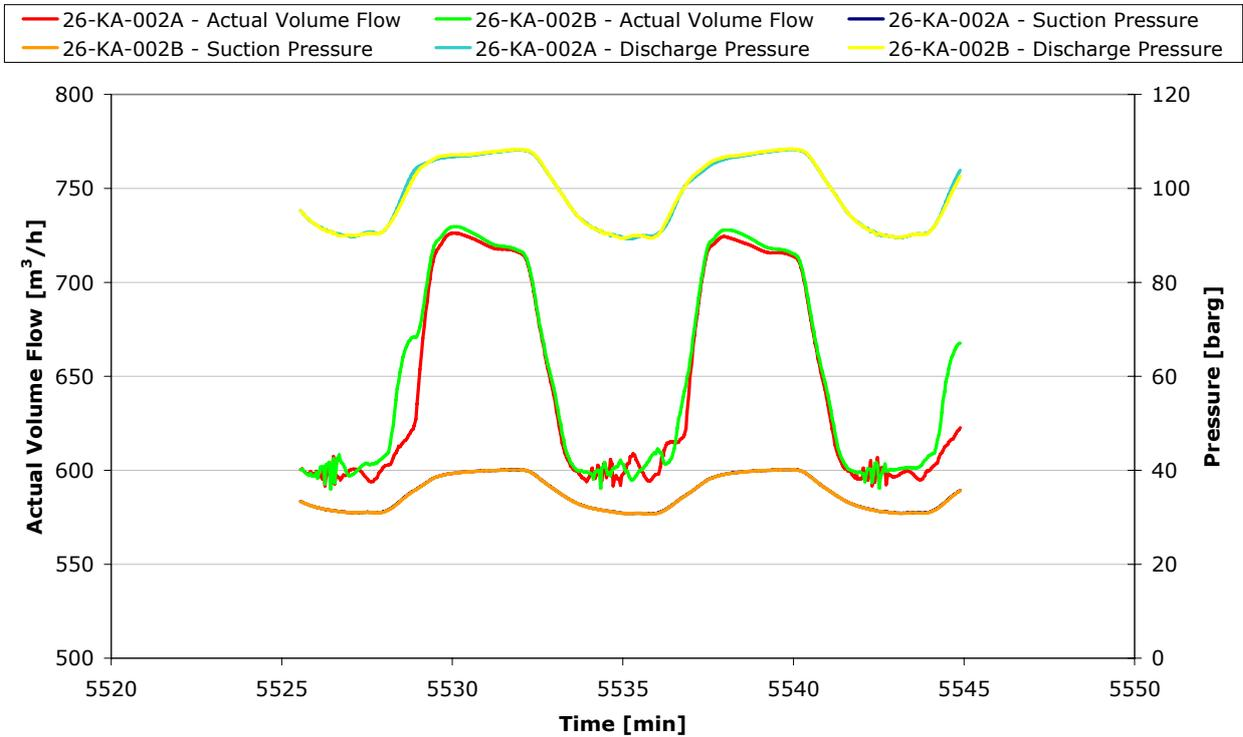
Figure 5.46. Actual volume flow, suction and discharge pressures for 2<sup>nd</sup> section compressors. Slug amplitude 50 % of normal flow and slug period 8 minutes.
