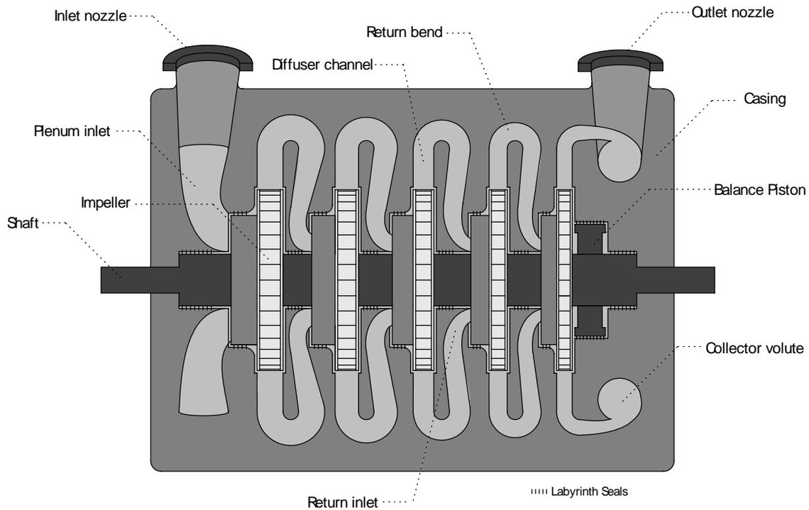
**Figure 2.1. Centrifugal Compressor with five stages.**
