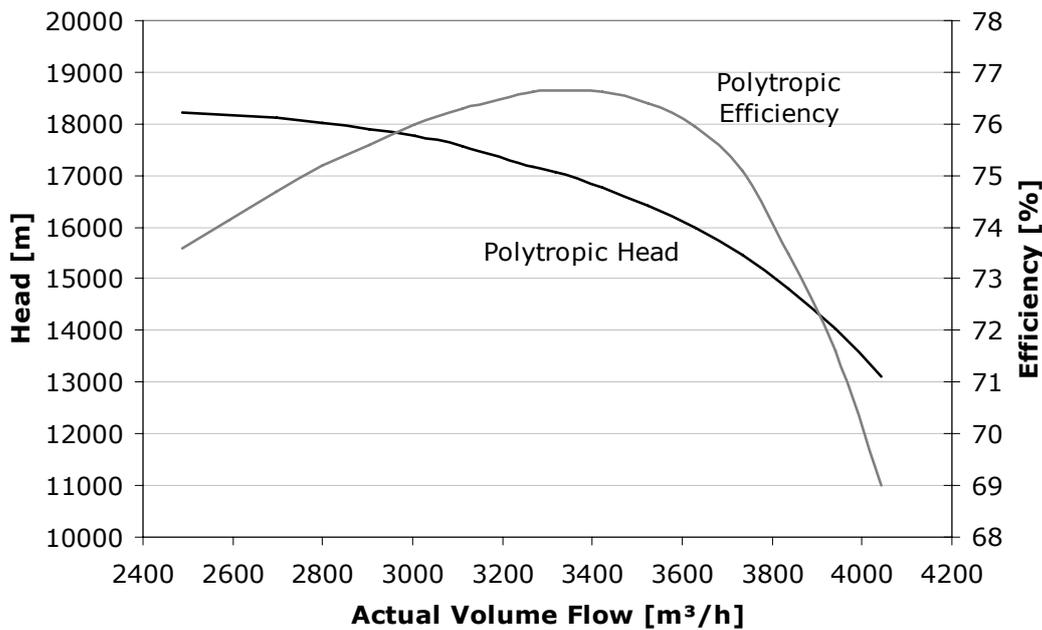
**Figure 2.9. Polytypic Head/Efficiency vs. Actual volume flow.**
