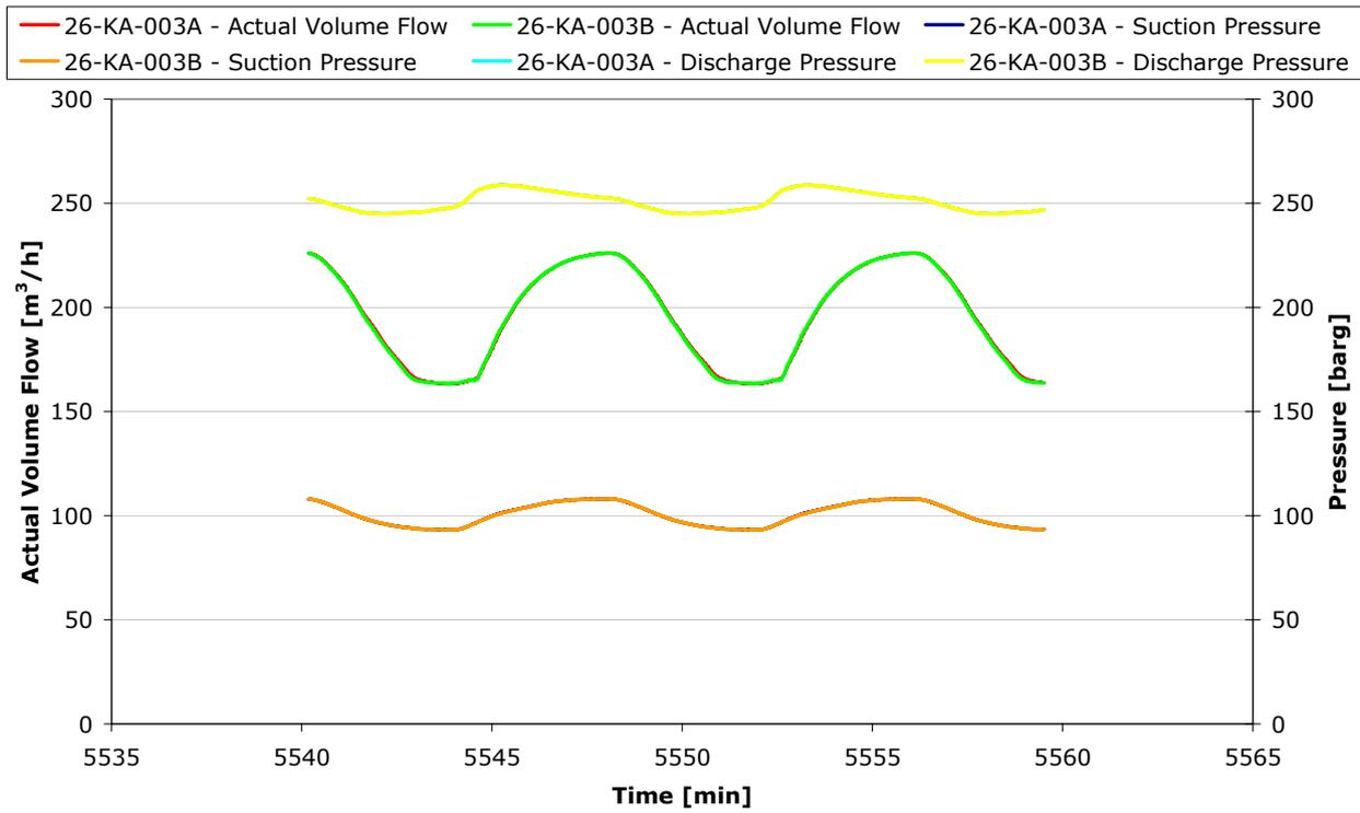
**Figure 5.44. Actual volume flow, suction and discharge pressures for 3<sup>rd</sup> section compressors. Slug amplitude 30 % of normal flow and slug period 8 minutes.**
