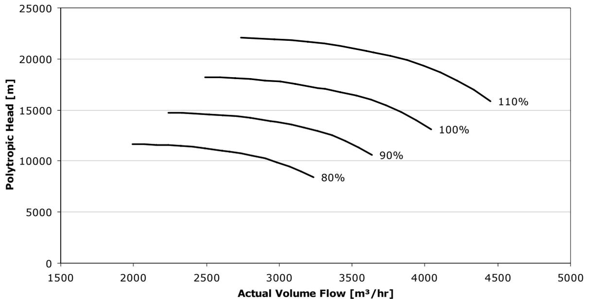
**Figure 3.18. Application of fan laws on the first section compressor curves of the OGPU at speeds of 80-110 % of design speed.**
