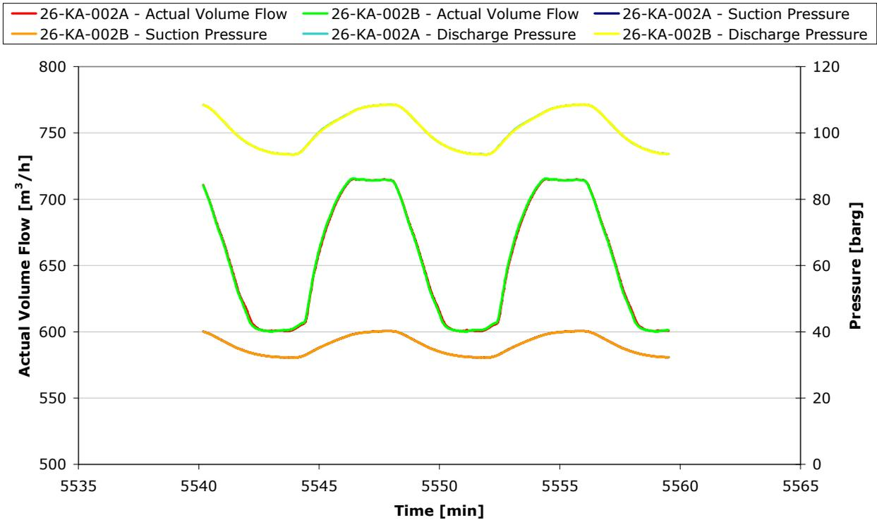
Figure 5.43. Actual volume flow, suction and discharge pressures for 2<sup>nd</sup> section compressors. Slug amplitude 30 % of normal flow and slug period 8 minutes.
