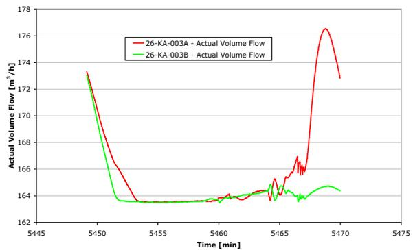
**Figure 5.40. 3<sup>rd</sup> section compressors inlet actual volume flows for the period of process oscillations.**
