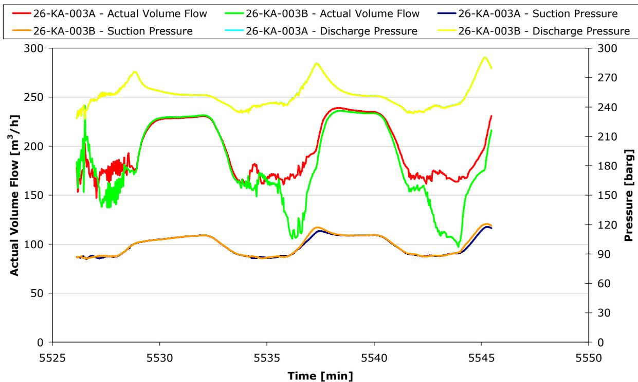
**Figure 5.50. Actual volume flow, suction and discharge pressures for 3<sup>rd</sup> section compressors. Slug amplitude 70 % of normal flow and slug period 8 minutes.**
