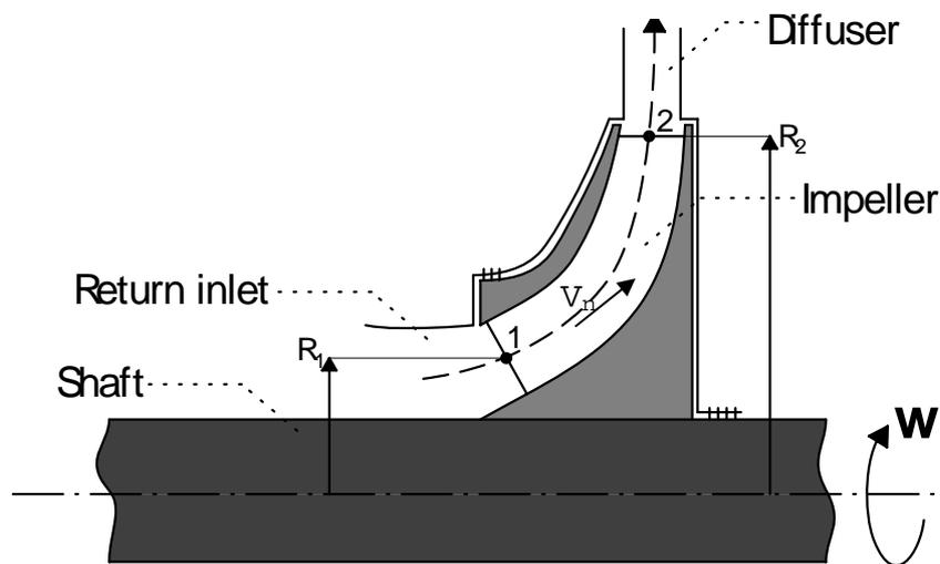
**Figure 2.4. Flow of gas through the impeller.**
