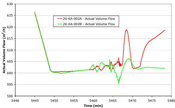
**Figure 5.39. 2<sup>nd</sup> section compressors inlet actual volume flows for the period of process oscillations.**
