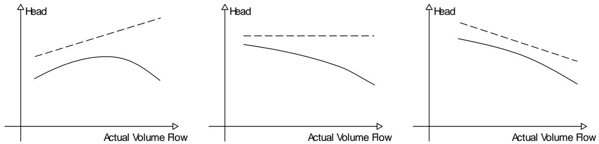
**Figure 2.6. Typical head curves (solid line) for the compressors with forward leaning, radial, and backward leaning impellers. The dashed lines are the ideal theoretical head curves for the zero inlet whirl situation.**
