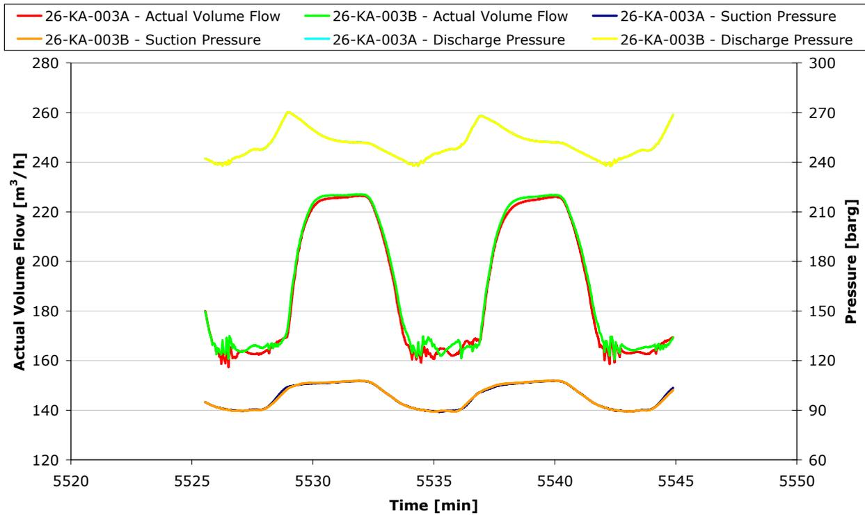
**Figure 5.47. Actual volume flow, suction and discharge pressures for 3<sup>rd</sup> section compressors. Slug amplitude 50 % of normal flow and slug period 8 minutes.**
