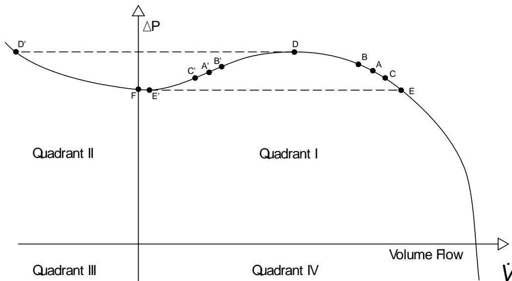
**Figure 2.15. Performance curve extended into the second quadrant. [Lüdtke, 2004]**
