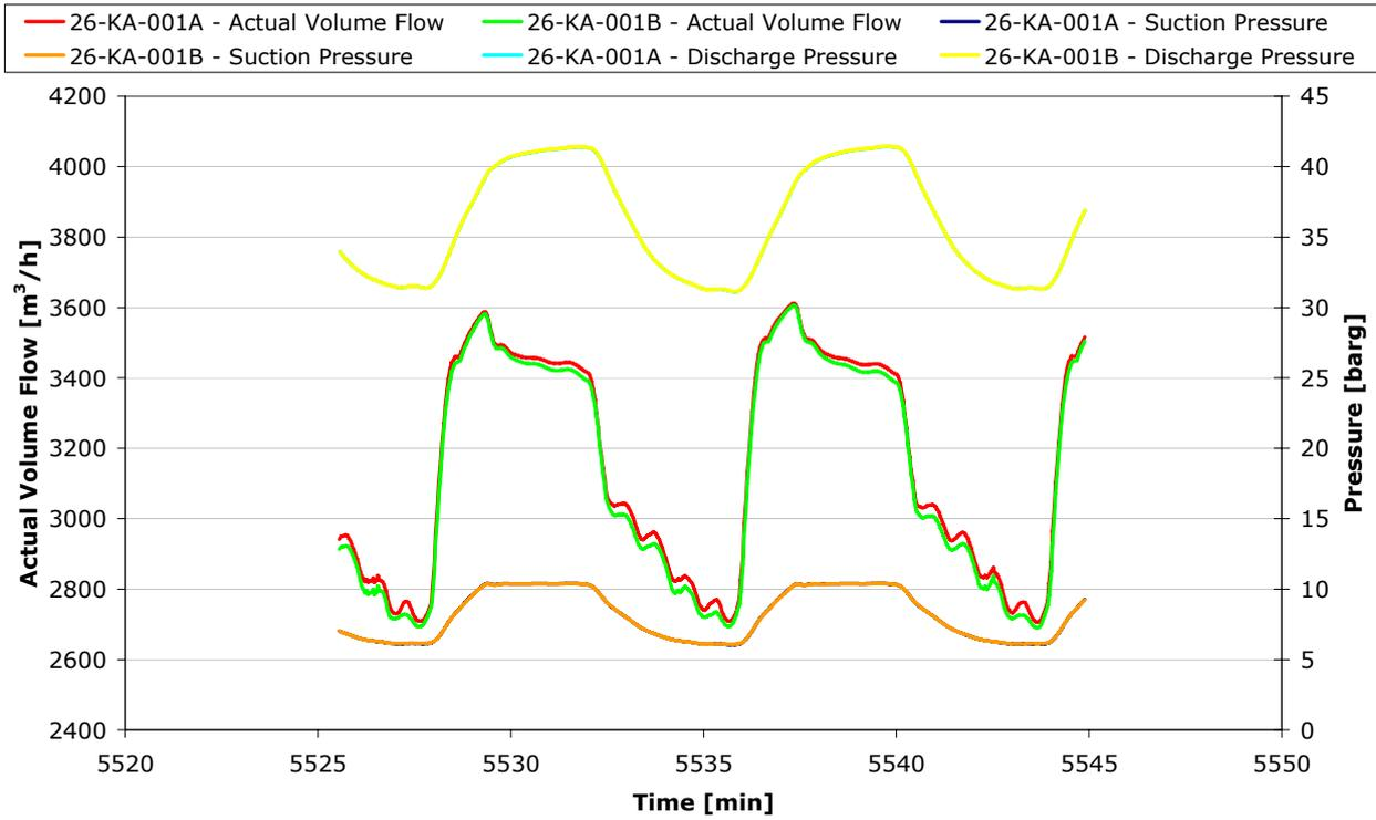
Figure 5.45. Actual volume flow, suction and discharge pressures for 1<sup>st</sup> section compressors. Slug amplitude 50 % of normal flow and slug period 8 minutes.
