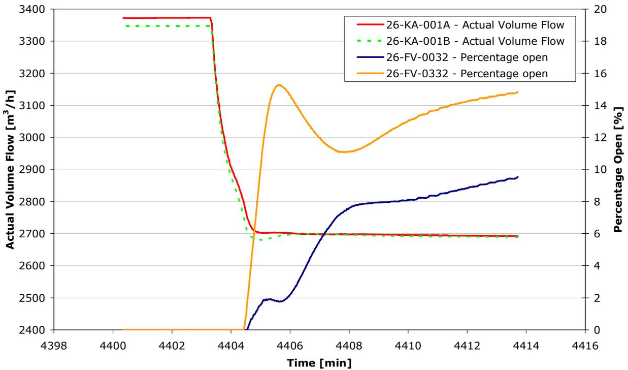
**Figure 4.29. Anti-surge control activation on 1<sup>st</sup> section compressors upon an inlet gas flow reduction to 50 % of normal flow.  $K_c=4$ ,  $T_i=0.1$  min, and  $T_d=0$ . Max. overshoot 10 %.**
