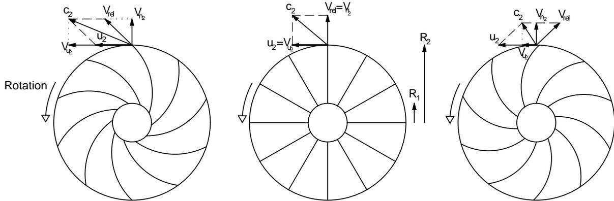
**Figure 2.5. Forward leaning, radial, and backward leaning impellers.**
