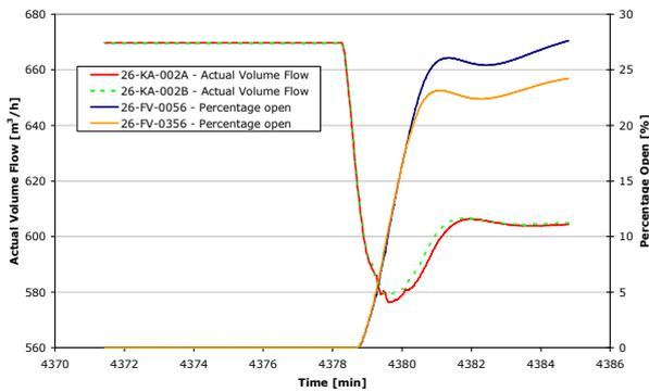
**Figure 4.27. Anti-surge control activation on 2<sup>nd</sup> section compressors upon an inlet gas flow reduction to 50 % of normal flow.  $K_c=0.5$ ,  $T_i=0.15$  min, and  $T_d=0$ .**
