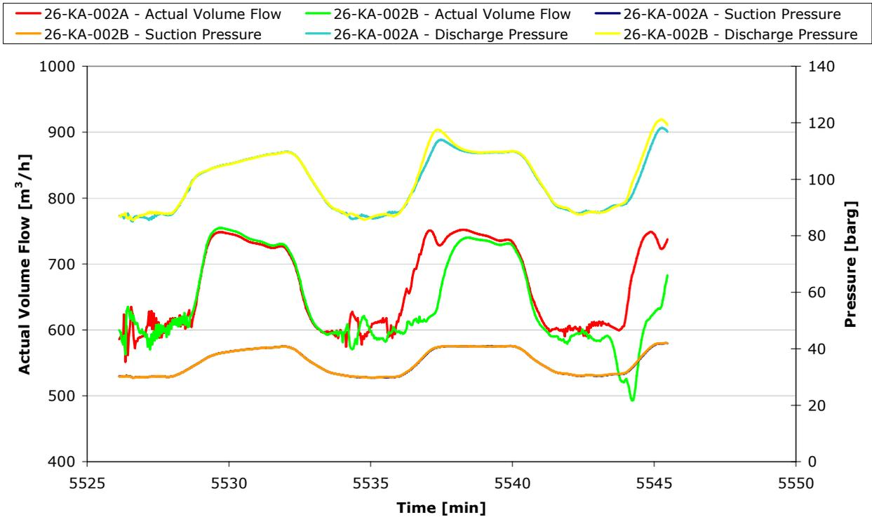
Figure 5.49. Actual volume flow, suction and discharge pressures for 2<sup>nd</sup> section compressors. Slug amplitude 70 % of normal flow and slug period 8 minutes.
