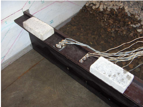
Figure C.29. Two concrete bricks placed on top of the platform in order to significantly change the eigen vibrations of the structure.
