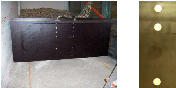
Figure C.4. Picture showing the wall placed in the wave flume and the two rows of strain gauges AA (left) and BB (right). To the right is a close up of three pressure transducers showing how they fit neatly into the wall surface.
