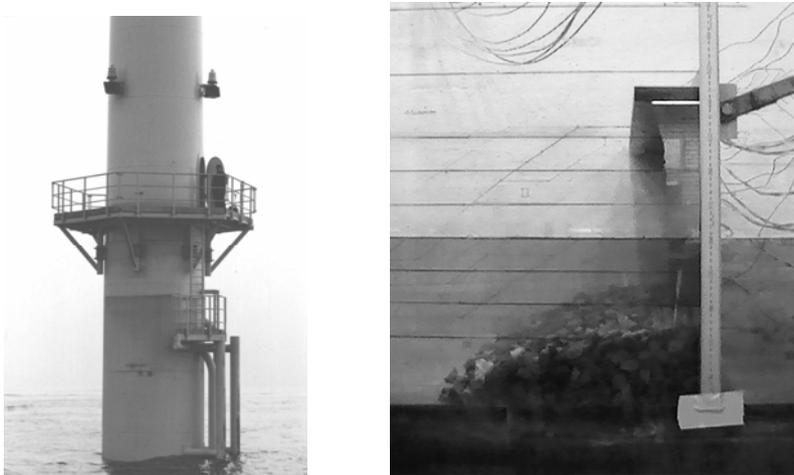
*Figure 6.1. To the left is the inspiration for the experiments depicted: A platform on the substructure of a wind turbine. To the right the simplified structure is used in the experiments depicted.*
