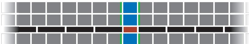
**Figure 10.14:** Insertion of a separation plane into the continuum model of Figure 10.12. The blue soil elements have no stiffness or mass, and the green line indicates elements with a “free” surface.
