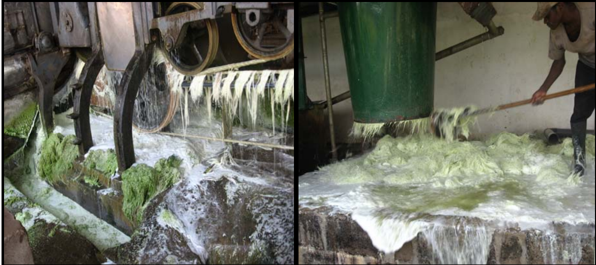
Photo 3.1 Decortication process and Flume Tow recovery
