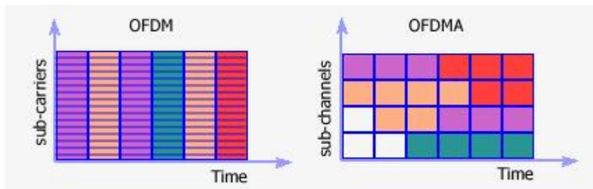
Figure C.2: OFDM/TDMA and OFDMA
