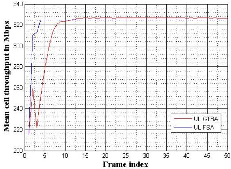
Figure 5.17: Mean cell throughput: GTBA vs FSA
