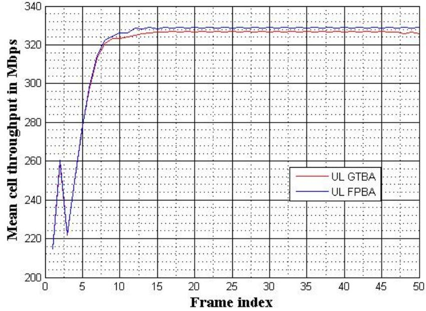
Figure 5.6: Mean cell throughput: GTBA vs FPBA
