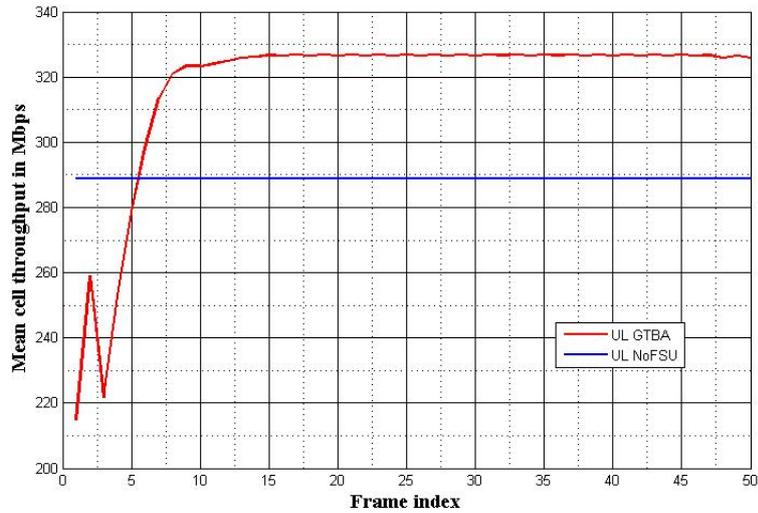
Figure 5.14: Mean cell throughput: GTBA vs NoFSU
