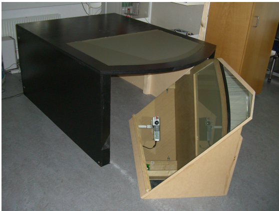
External view of the demeTouch table. The main component we can see on this picture are the mirror and the screen area on the top of the Table.
