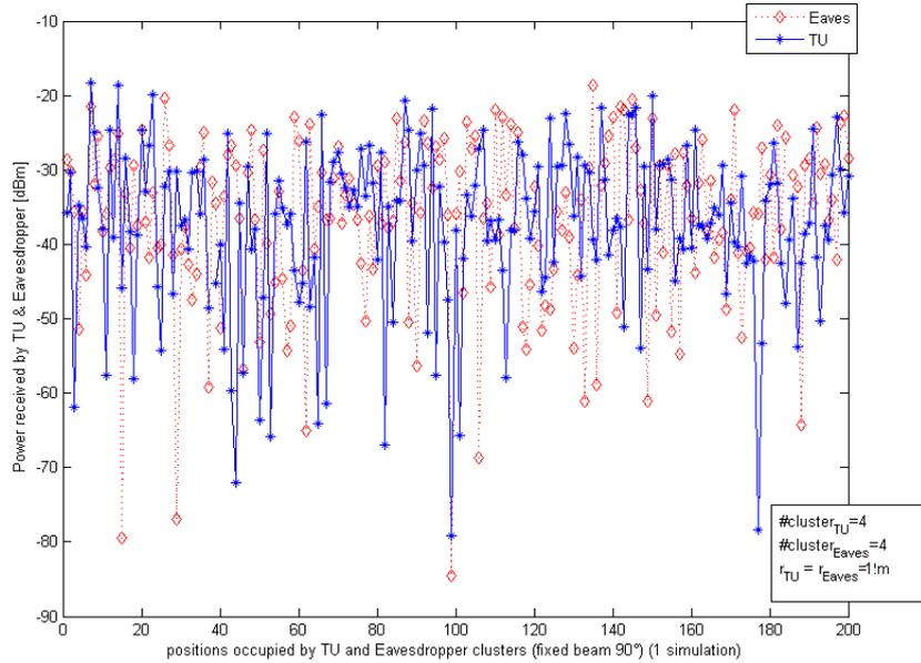
Figure 4.6: Power received by the target user and the eavesdropper after 1 simulation ( $90^\circ$ )
