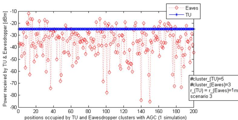
Figure 4.20: Power received by both TU and Eavesdropper over 1 simulation (5cl vs 3cl)
