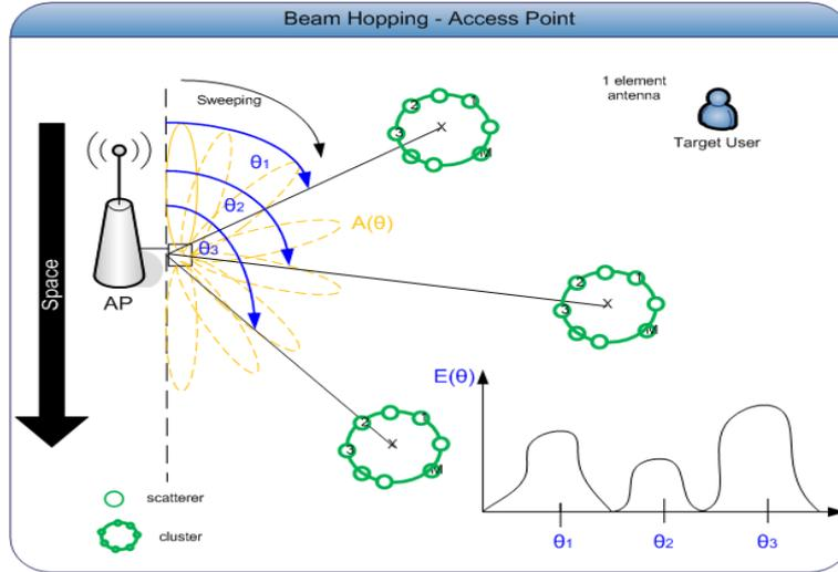
Figure 1.5: Beam Hopping applied by AP
