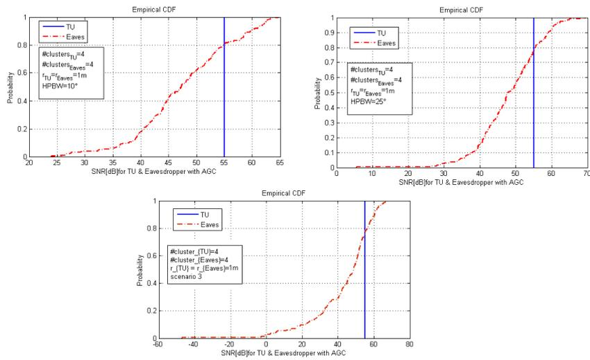
Figure 4.36: CDF of the SNR with a HPBW of  $10^\circ$  (top left),  $25^\circ$  (top right) and  $60^\circ$  (down)(scenario 3)
