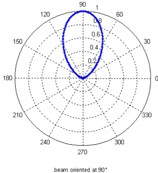
Figure 4.2: Fixed beam oriented in the 90° direction
