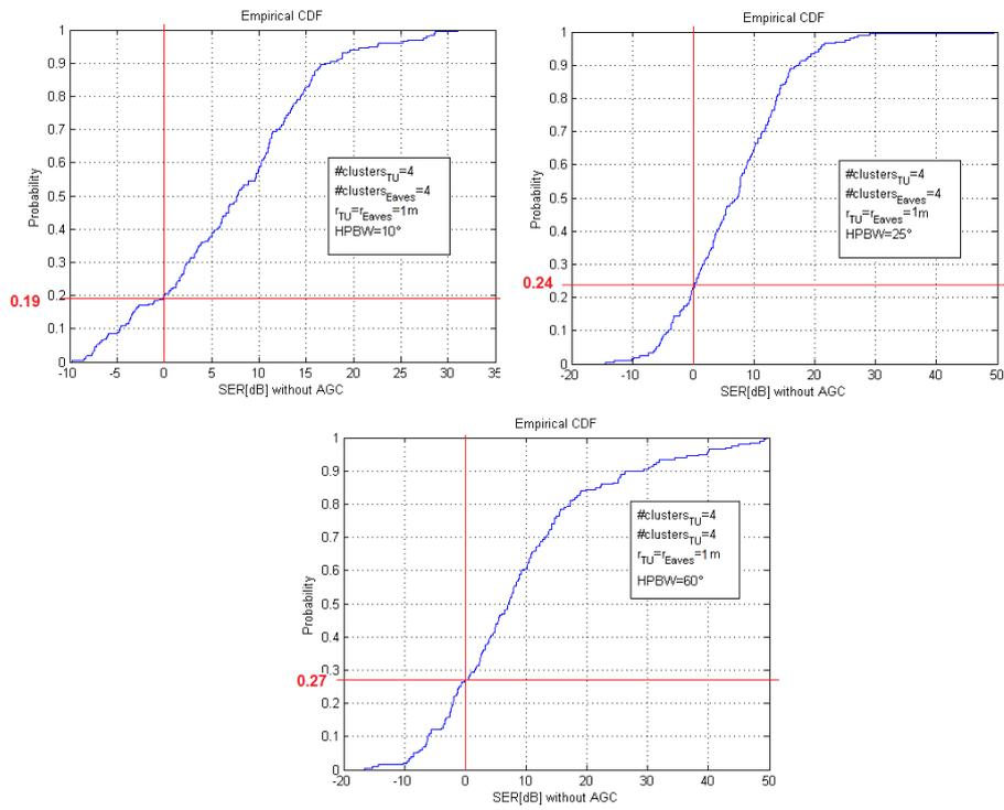
Figure 4.35: CDF of the SER with a HPBW of  $10^\circ$  (top left),  $25^\circ$  (top right) and  $60^\circ$  (down) [dB]
