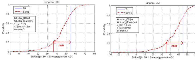
Figure 4.33: CDF of the SNR [dB] comparison between the radius in scenario 3 (4cl vs 4cl)
