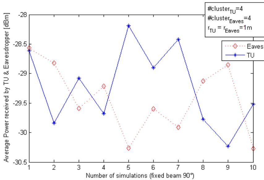
Figure 4.4: Average power received by the target user and the eavesdropper after 10 simulations (90°)
