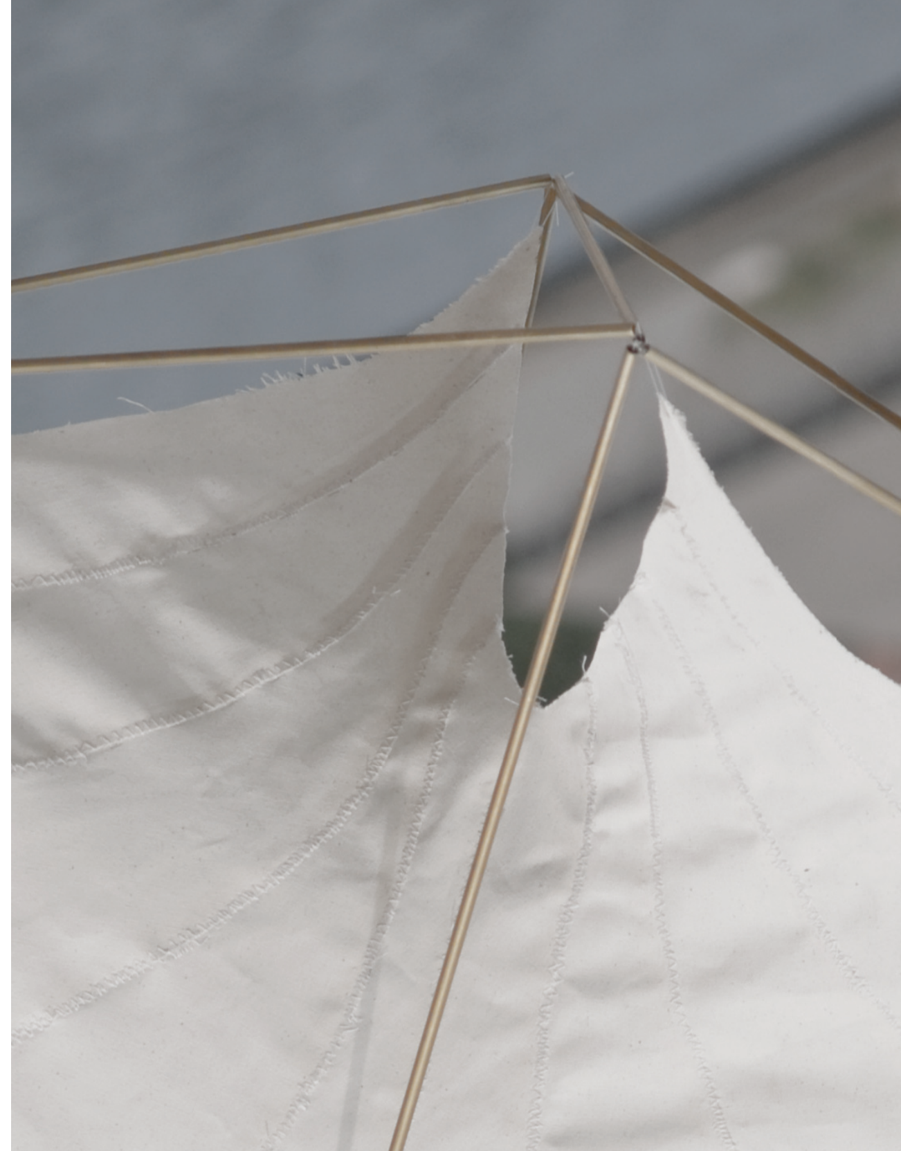
Above: Test of pretensioned membrane manufacturing
