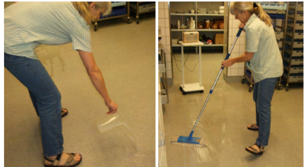
III 32 | Cup method: A cup of soap-water is splashed on the floor and dry mops are used to wipe off.
