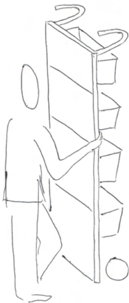
ill.49 | Slim: This cart has a very slim structure when folded and appears as a very closed and clean object that can be stored visible for clients/customers. The folding principle is complex and probably not easy.
