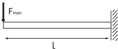
III. 16.11 | Forces and dimensions on cart
