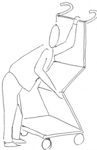
ill.49 | Slim: This cart has a very slim structure when folded and appears as a very closed and clean object that can be stored visible for clients/customers. The folding principle is complex and probably not easy.
