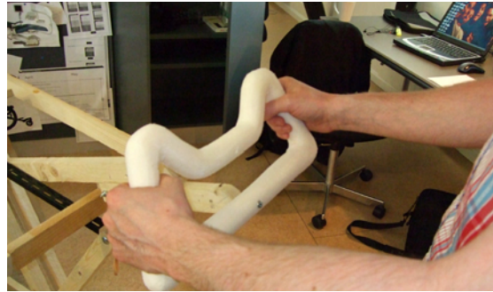
Ill 89: Model 3 is similar to model 2, but it is shaped so that the handle can be folded down in the buckets, when the cart is folded. The handle is big and has as model 2 many areas that can not be used.
