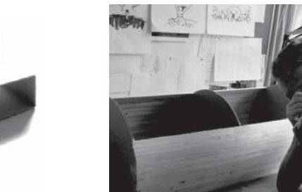
Concrete model construction process. Photo. The barrel form serve as inside form work of 1:20 concrete model.
