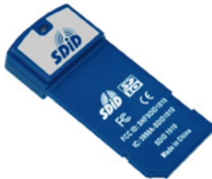
ill. 30 The card which makes it possible for the PDA to read RFID tags
