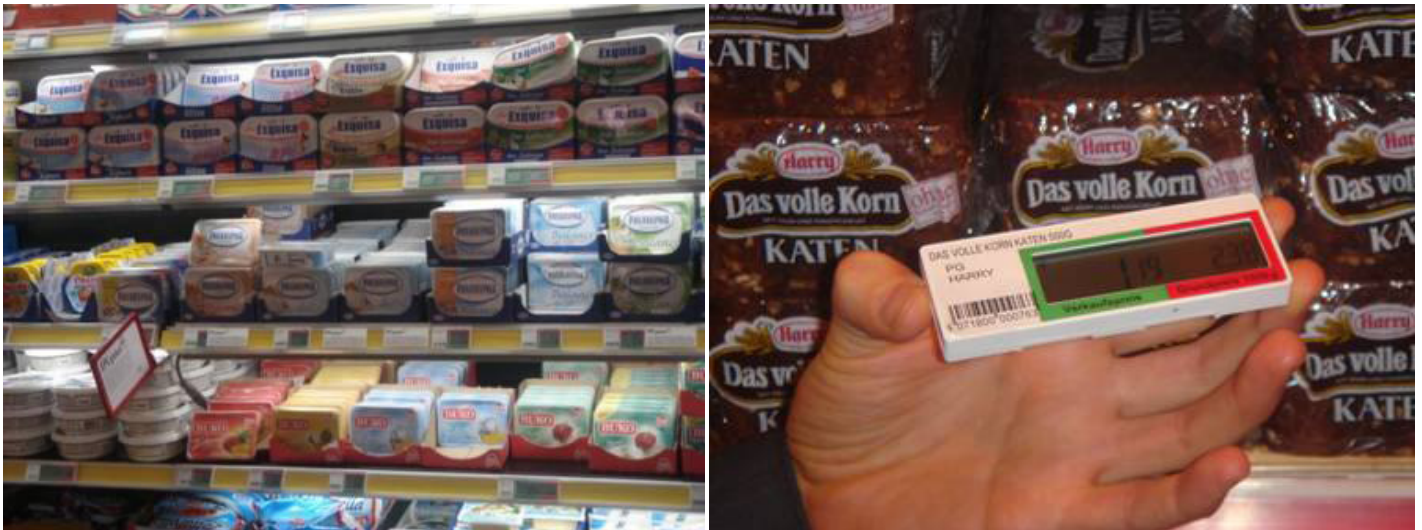
ill. 29 Smart shelves hold RFID tagged product and notify the stockroom when more products are needed.
