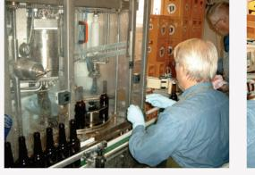
The conveyer belt transport the bottles to a machine where the beer is filled in and
