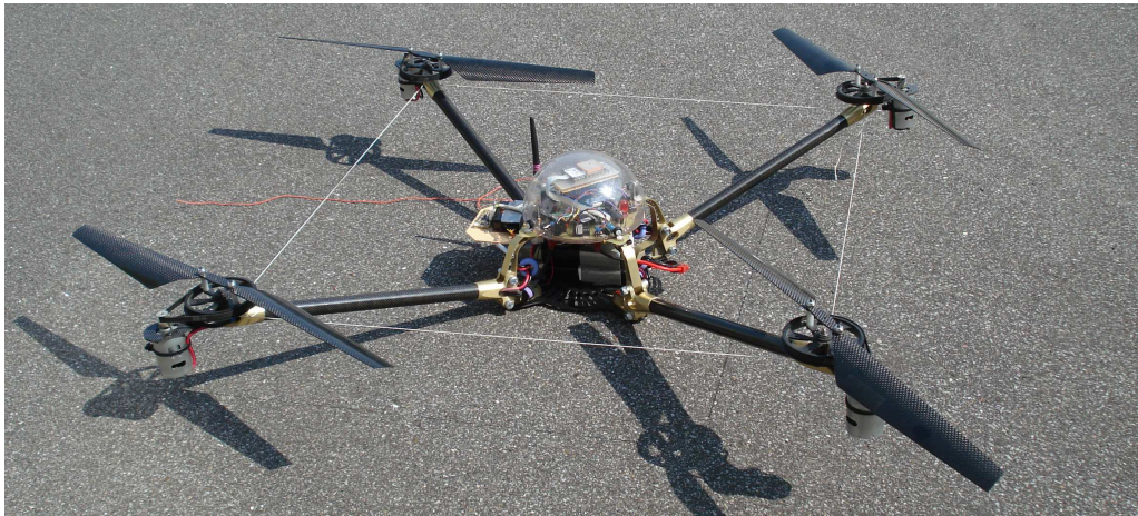
PICTURE 2.1: The final hardware platform fully equipped with sensors, total weight is 2.6 kg.
