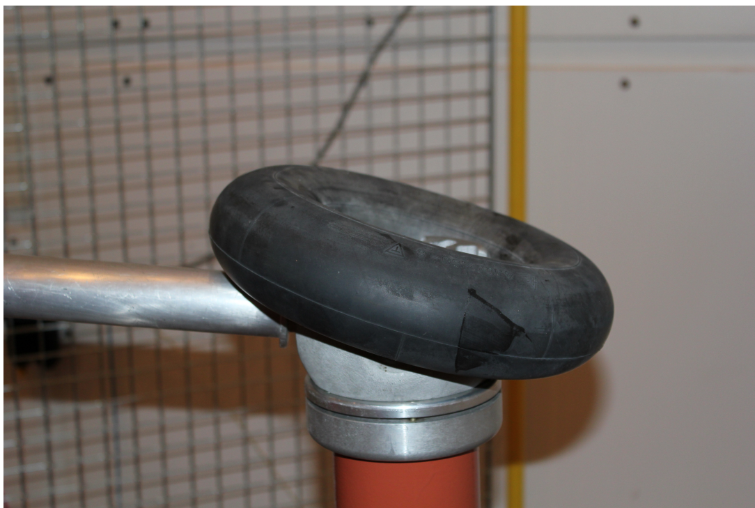
Figure 3.15: The rubber tube that is placed on the sphere.
