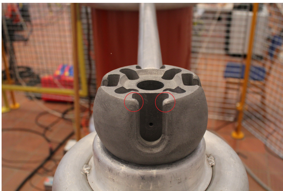
Figure 3.13: The red circles indicate where the PD occurs on the sphere.
