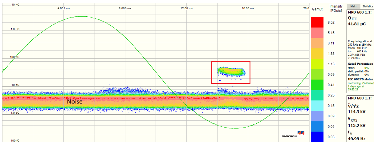
Figure 3.11: The PD starts at 114.2 kV. The red square marks the PD pulses.
