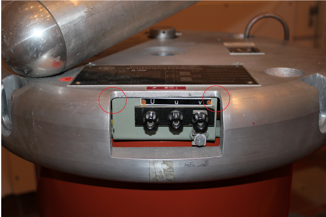
Figure 3.18: The placement of the PD activity on the transformer is marked with two red circles.
