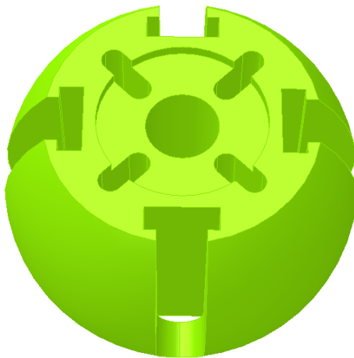
(a) The connecting sphere modeled in Opera3d.
