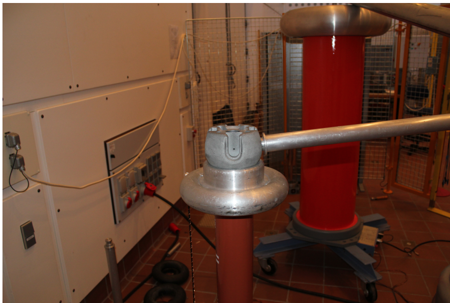
Figure 3.12: The connecting sphere where the PD activity occurs.
