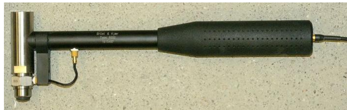
Fig. 3.3: B&K 8202 hammer used in the modal experiments.
