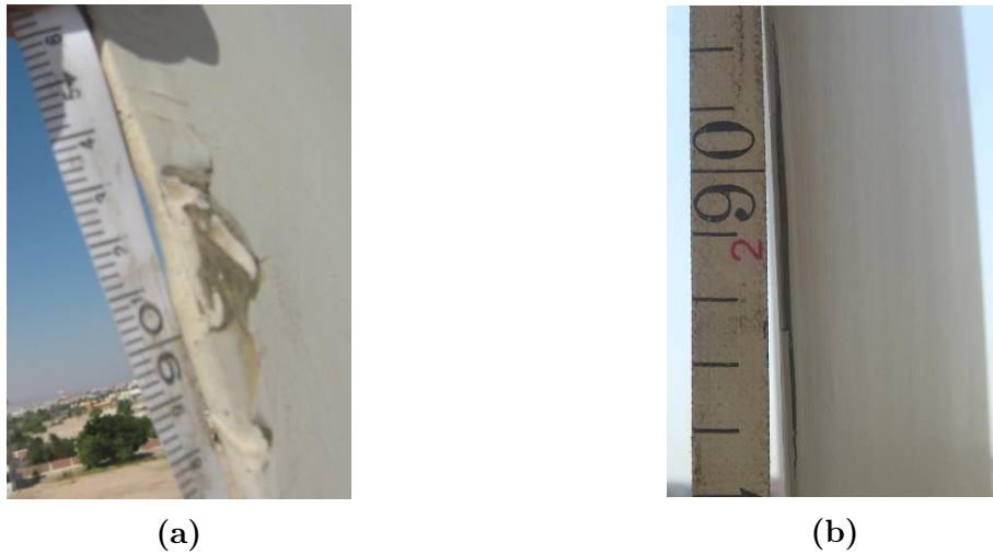
Fig. 1.5: Edge damages in wind turbine blades [9]. (a) Edge crushing. (b) Debonding.
