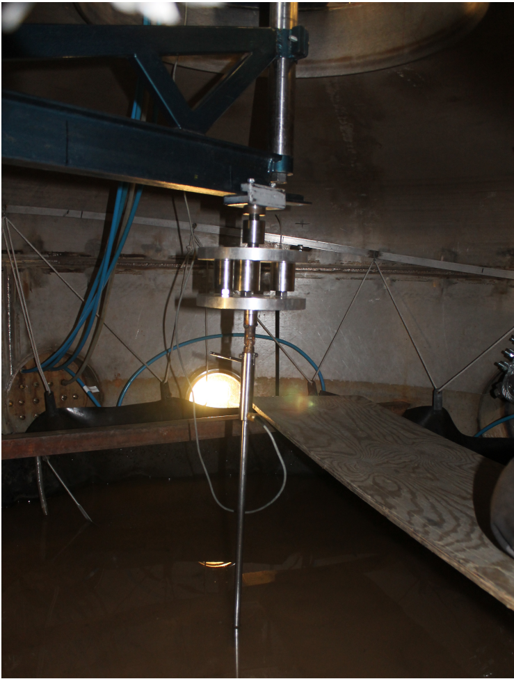
Figure H.6. The CPT equipment mounted and ready for test in the center of the tank.
