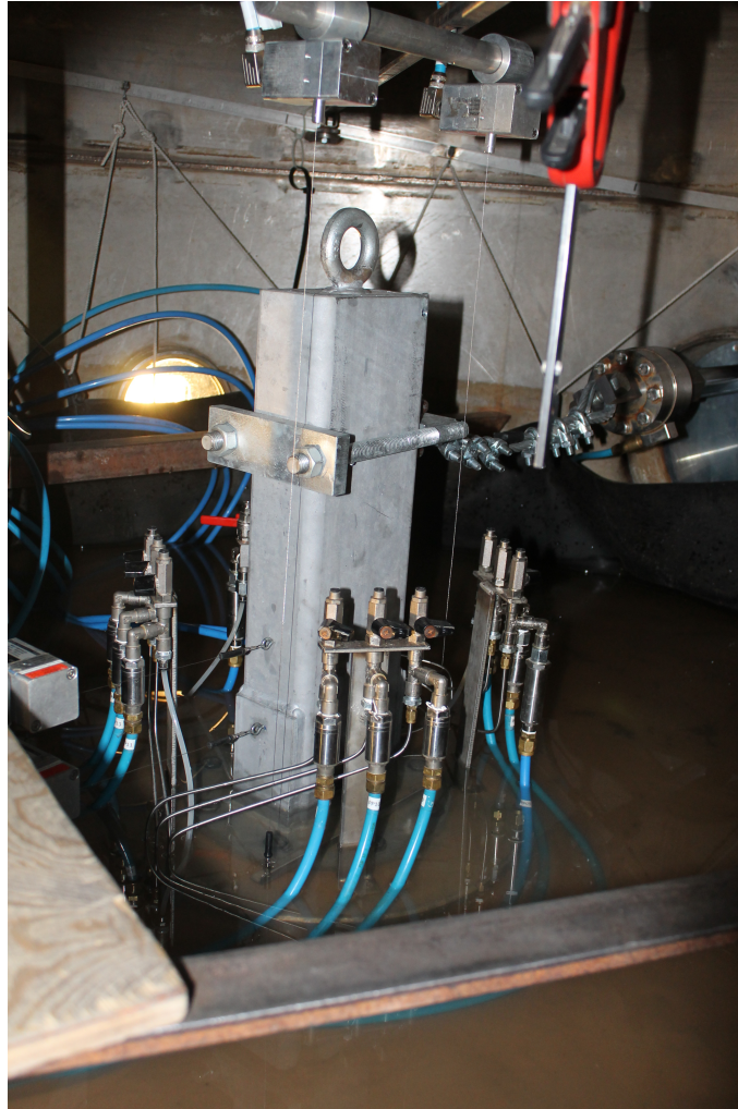
Figure H.10. The installed bucket with the displacement transducers visible.
