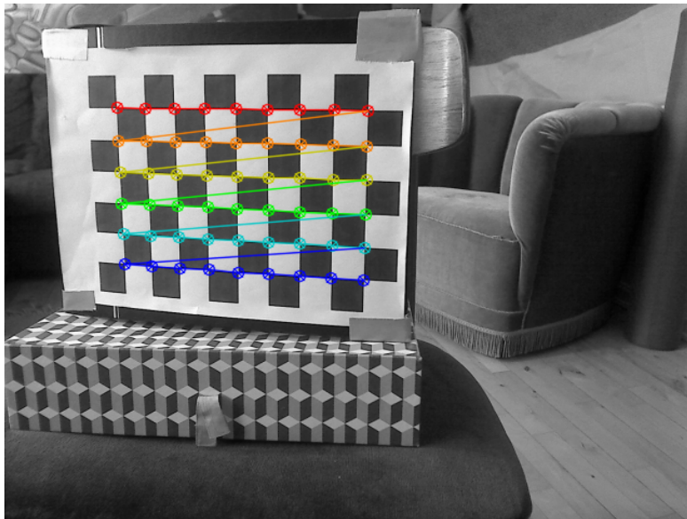
Figure 5.2: Calibration image with checkerboard corners shown found by cv::findChessboardCorners . The image is produced with the function cv::drawChessboardCorners .
