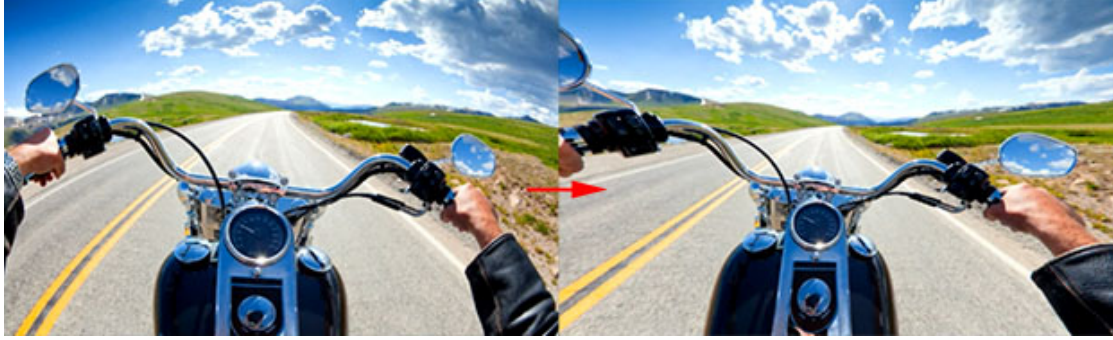
Figure 2.4: The lens distortion is corrected from the left to the right image. This for example be seen on the edge of the road [8].
