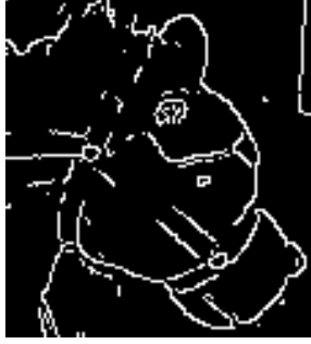
Figure A.11: Output from the Canny edge detector with thresholds 220 and 200
