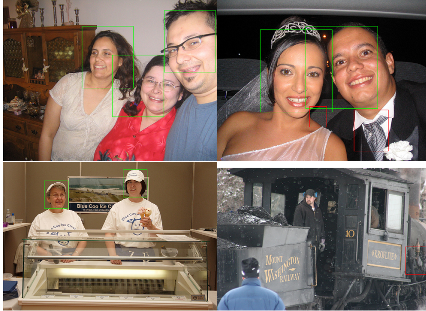
Figure 3.11: Examples of output images from the HOG detector where all data sets were used for training. Valid and invalid matches are indicated by green and red rectangle respectively.
