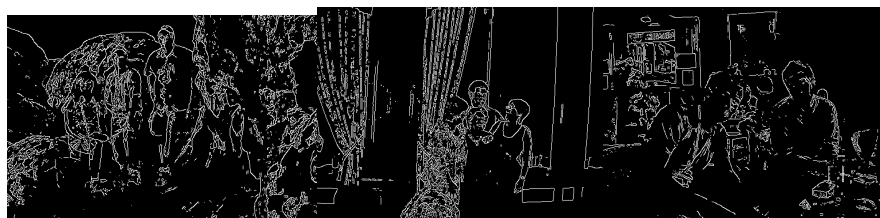
(d) Canny edge detector with thresholds 200 and 180
