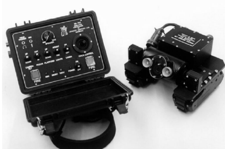
Figure 2.1: The Inuktun Microtracs robot [12]
