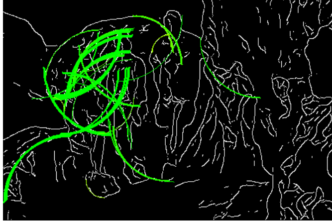
Figure C.2: Results of using equalization to balance the out the responses. It is apparent that larger shapes are now dominating and producing erroneous matches.
