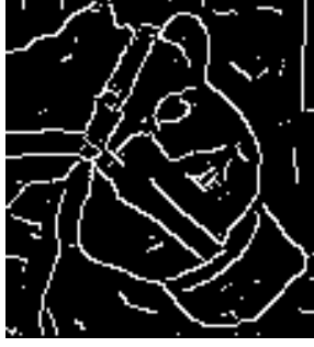
Figure A.14: Edge map obtained by applying the Pb detector
