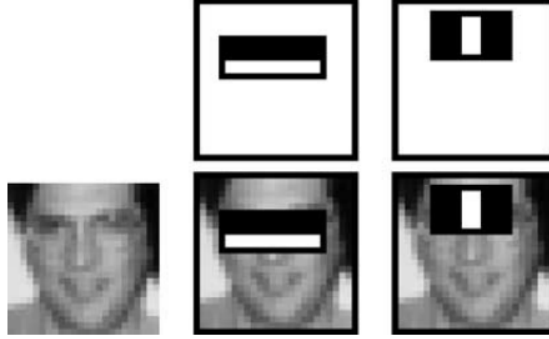
Figure 2.7: Example of Haar-like features used in face detection [45]
