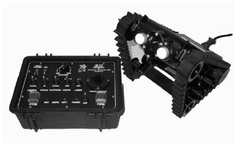
Figure 2.2: The Inuktun MicroVGTV robot [12]
