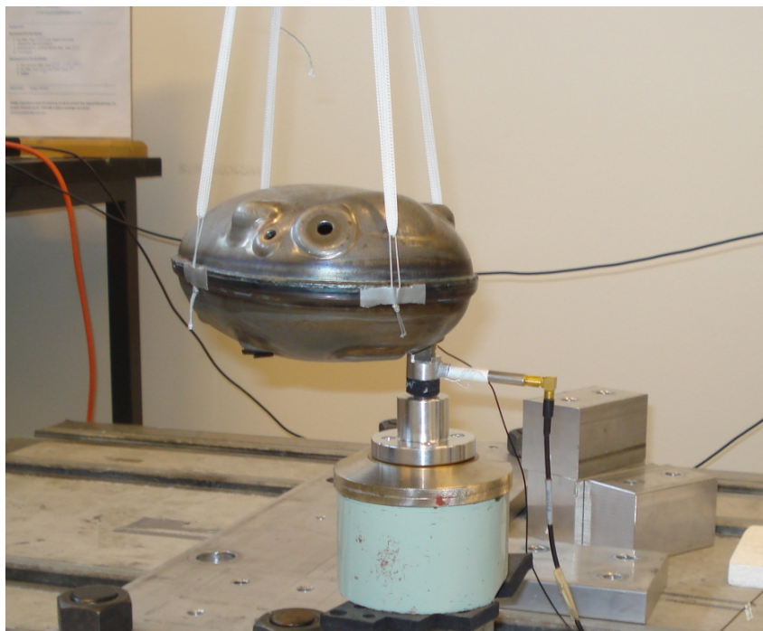
Figure 5.1: Picture of experimental set-up; pure housing suspended on four rubber bands and acoustic exciter with adaptor m#3.
