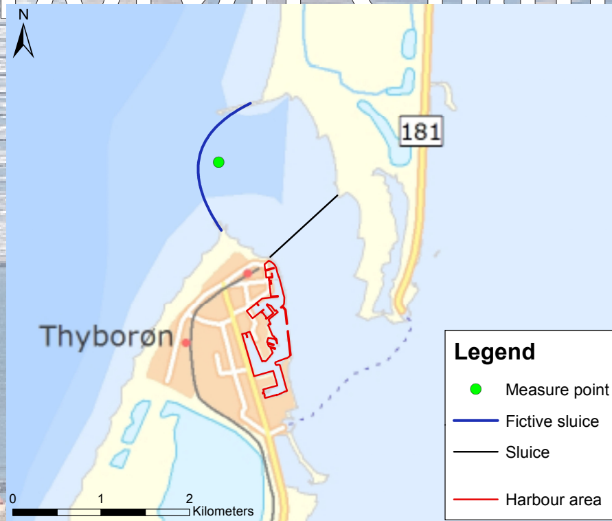
Figure 6.2: Sketch of the intended and model location for the sluice and the measuring point.
