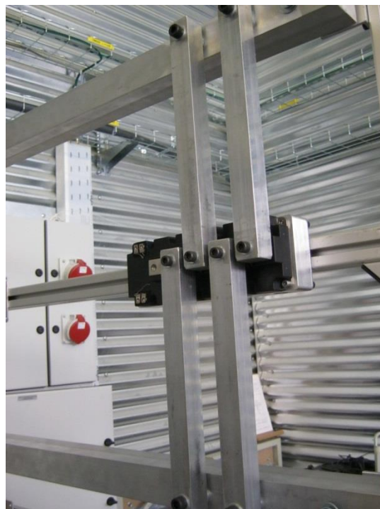
Fig. 2.26. Picture of the IGBT diagonal electrical connections in order to have an easy and variable connection for the cooling items
