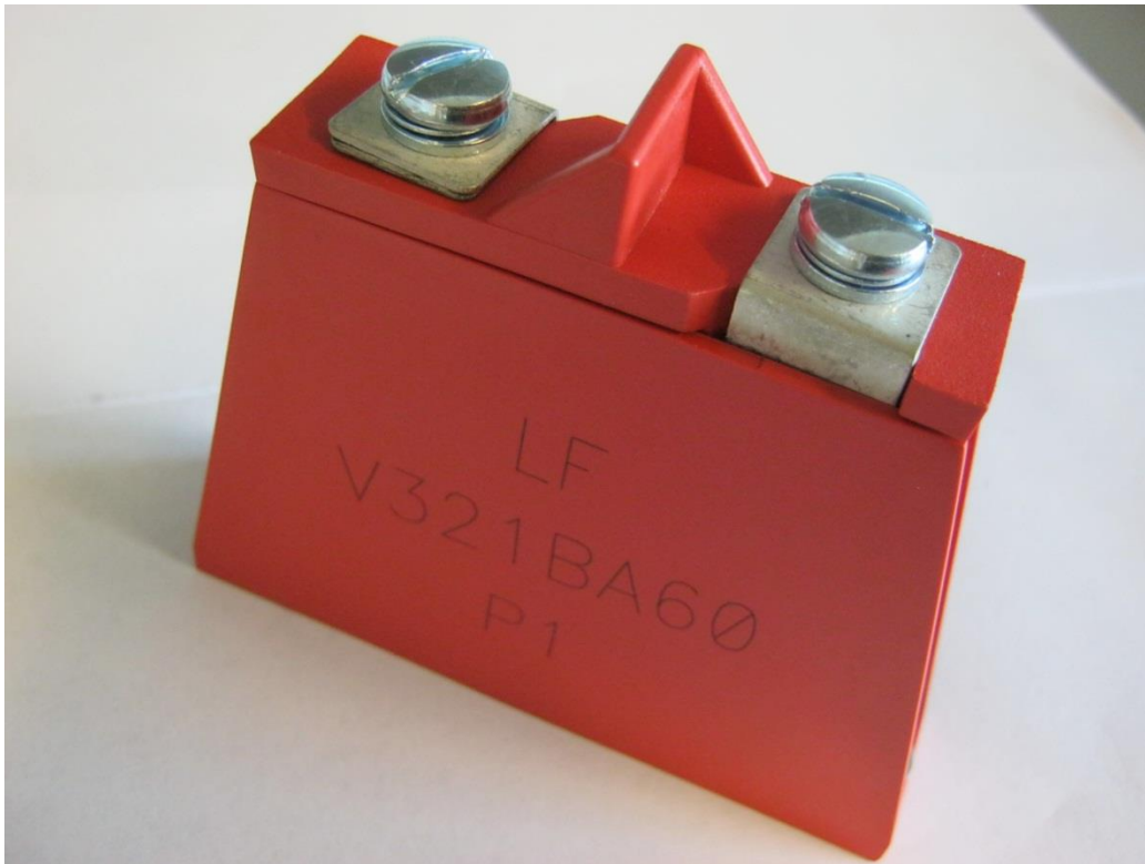
Fig. 2.15. Picture of the Varistor used on the DC-link side for surge protection of the IGBTs
