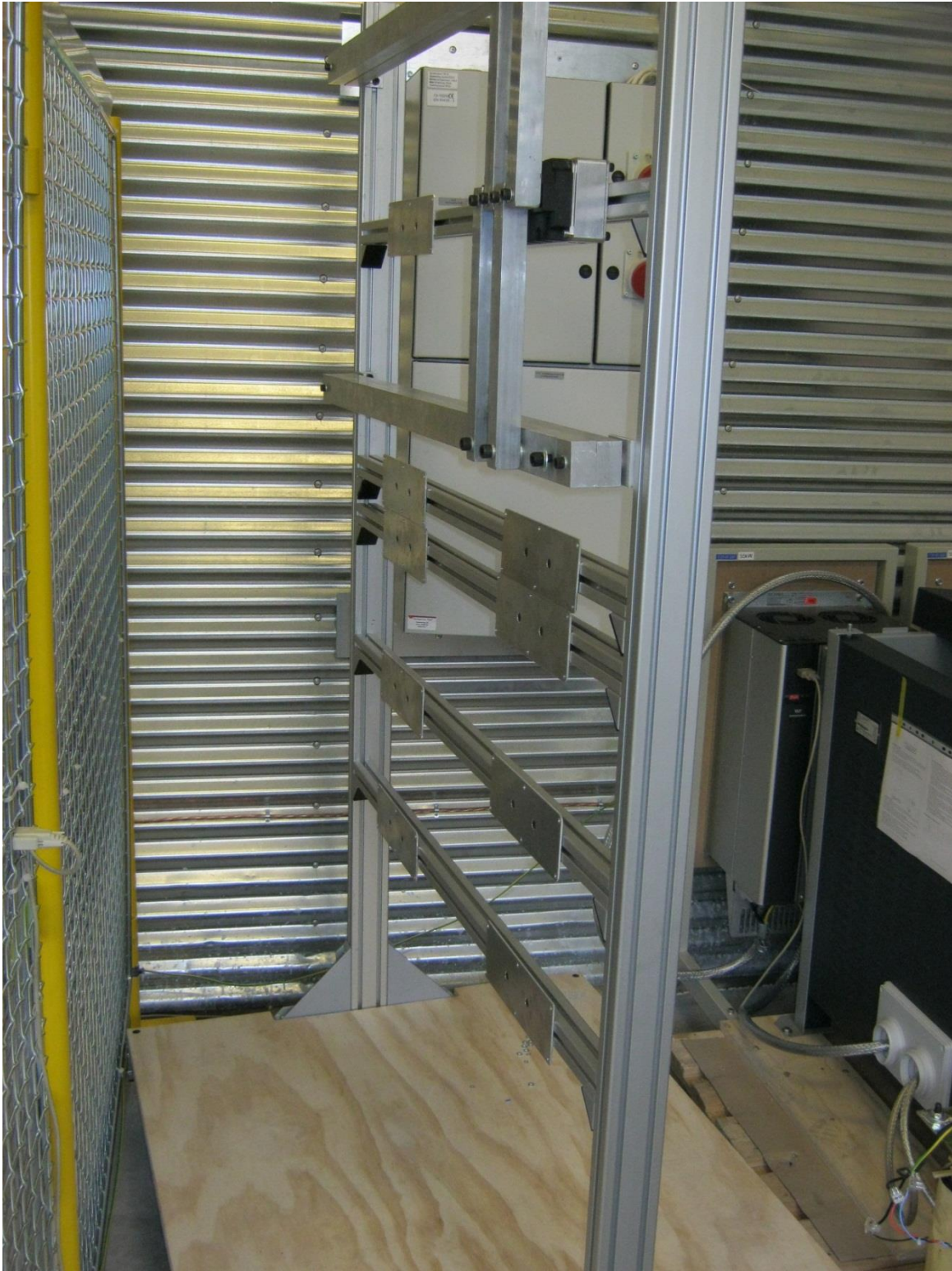
Fig. 2.24. Picture of testing IGBT power module chassis for an easy connection between their electrical and cooling parts
