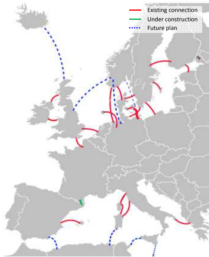
Figure 1.2 - HVDC connections in Europe [10]
