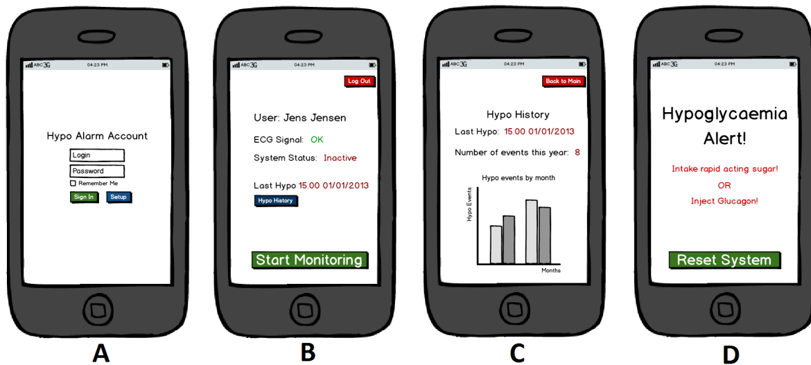
Figure 7.3: System Mock-up, first iteration. A: Login screen, B: main screen, C: hypoglycaemia history screen, D: hypoglycaemia alarm screen
