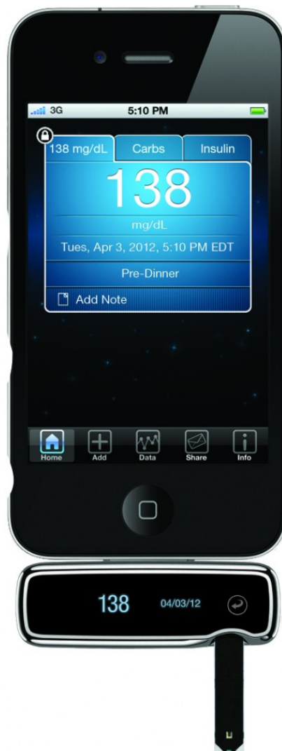
Figure 1.4: iBGStar glucose monitor is connected with a smartphone. A test strip is inserted directly into iBGStar.
