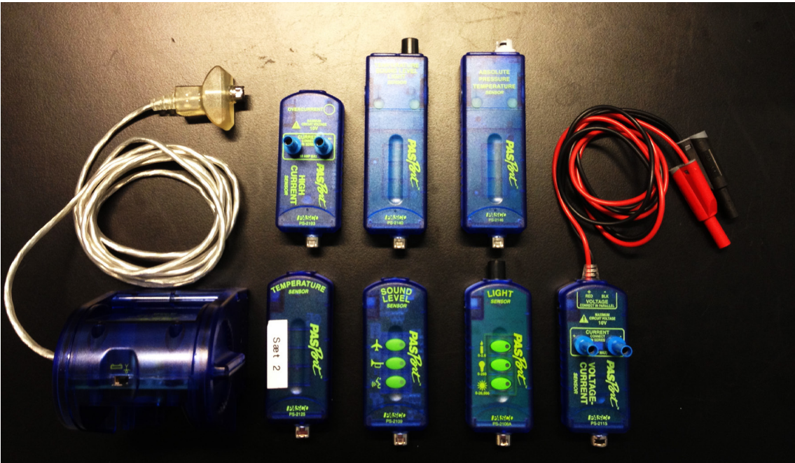
Fig. 23. 'Pasport' sensors, Left to right bottom row: Distance, temperature, sound level, light, voltage. Left to right top row: Current, Chemistry Sensor, Physics Sensor.
