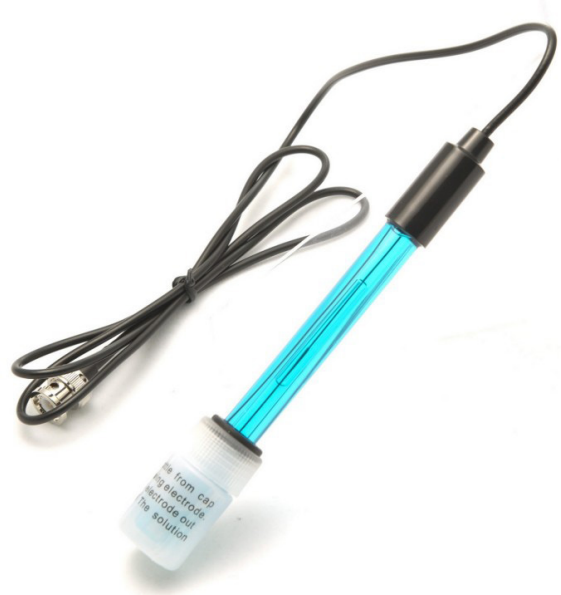
Fig. 40. A standard pH sensor which would be bought for a pH-meter. This would with the BNC connector be possible to use this probe with almost any pH-meter.
