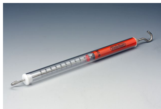
Fig. 13. A newtonmeter which could be used to perform an experiment with friction, but it would be much harder to get accurate data and thereby understand the theory of friction..
