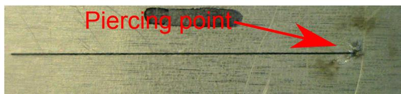
**Figure 10.4:** Example of an experiment showing that no HAZ occurs but that spatter (the brownish color) occurs around the piercing point.
