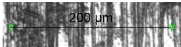
**Figure A.4:** The ruler from the microscope picture is used to find the pixel  $\mu\text{m}$  ratio. The green areas shows the two chosen pixels, which measures the number of pixels used for calculating the ratio. The ruler is 453 pixels.
