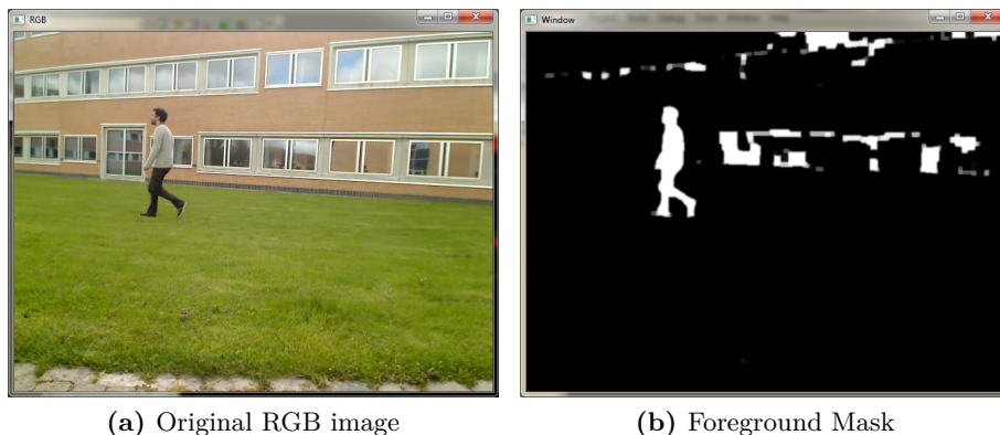
Figure 3.10: Illumination problems at optimal parameters.
