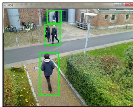
Figure 2.32: Gauss Mixture Model Limitations. Two persons in the scene are detected as one blob
