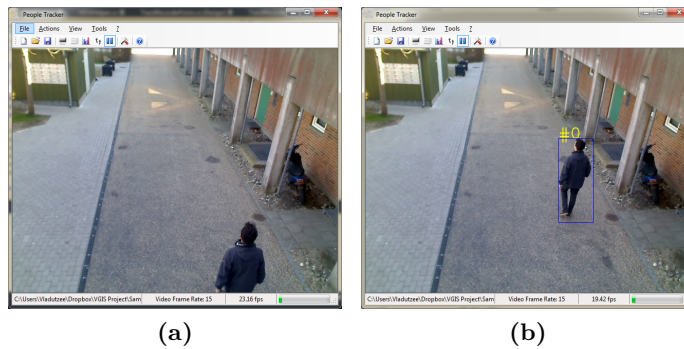
Figure 5.1: Detection/Tracking done only when the entire human blob appears in the scene.
