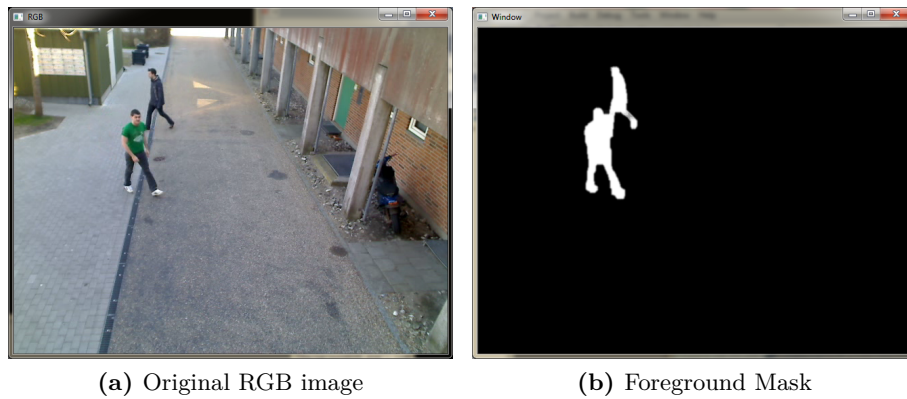
Figure 3.13: Background subtraction. Totally shaded environment
