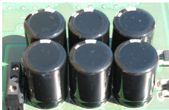
Figure 4-2 – DC Link Capacitors from the Developed Experimental Board
