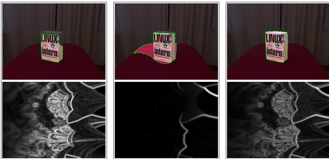
(a) An edge map based on color only. (b) An edge map based on depth only. (c) A mixed edge map with a color-depth ratio of 3:2.
