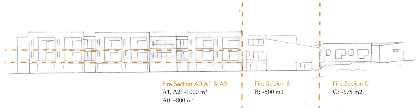
III. 7.4.1 Fire Sectioning
