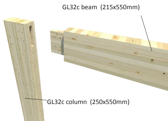
III. 3.16 Connection Nr.1 Plug-in connection between column and beam, which are fix together with bolts.
