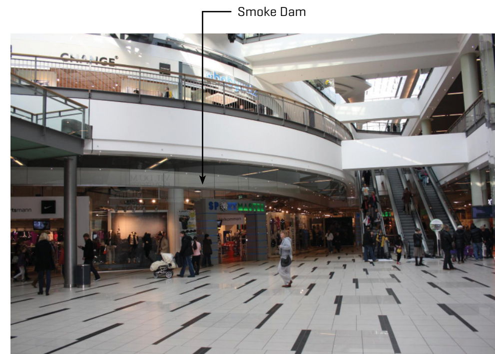
ill.119 Smoke dams sit below the floor to channel the smoke out and away from the emergency exits.
