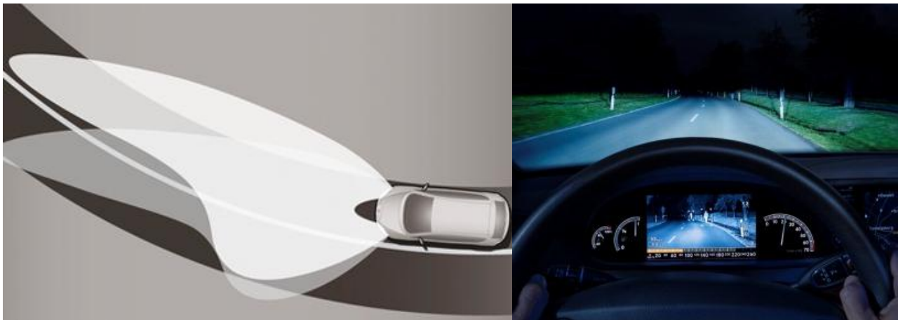
Figur 5 : Tv. Adaptive Frontlights - Kilde: Seat Automotive 20 Th. Night vision system – Kilde: Bosch Group 21
