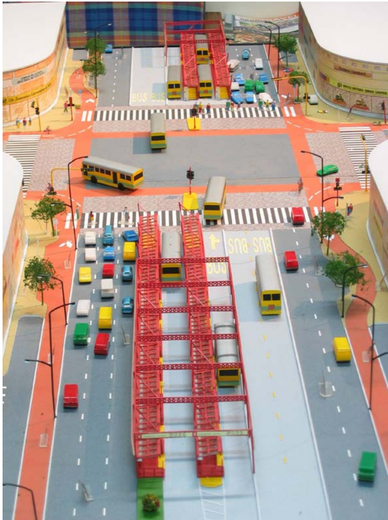
Figure 4.9: Model of the principle for the proposed layout of the HCBS. The bus stops are placed before the intersection between the car lanes. (Photo: Sriram Bhamidipati, TRIPP)
