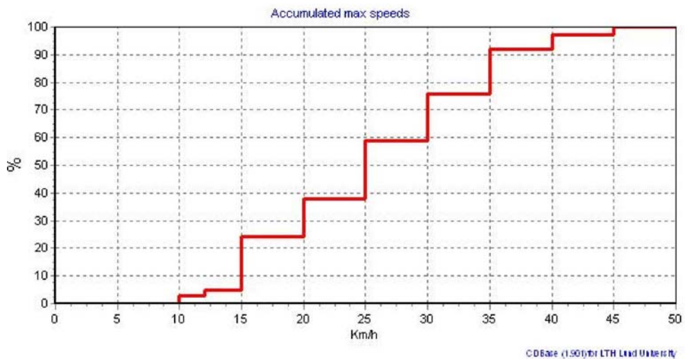
Figure 3.5: Accumulated max speed of the two road users involved in a conflict (only serious conflicts according to CDBase definition)
