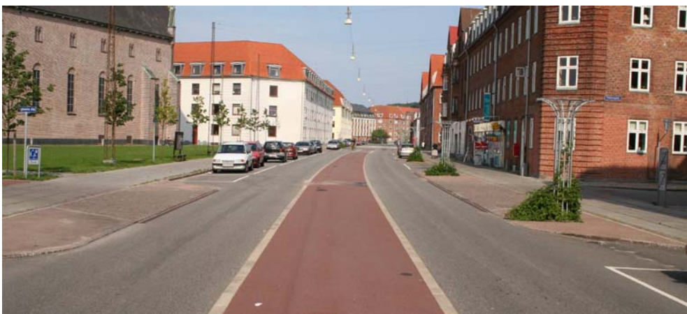
Figure 4.7: Narrowing – a passable middle island at a local road in Aalborg, Denmark.
