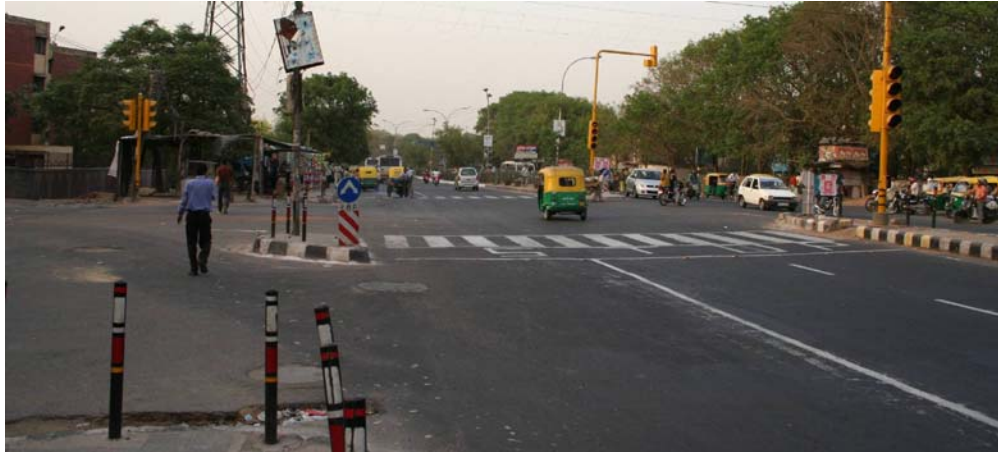
Figure 2.7: Photo towards north at Orthonova. Notice the "shunt" lane to the left that merges with the service lane. The northbound lane has one bus lane and two car lanes.
