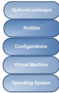
Figure 3.9: CLDC Configuration Architecture
