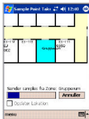
Figure 8 PocketPC Sample Point Taker showing how teach-points are being collected
