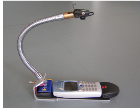
Figure 3: The mini-camera with the mobile barcode scanner system attached.
